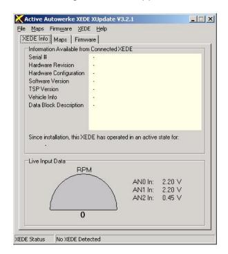
The Xede software will try to automatically connect and communicate with the processor, if successful then the above blank box will display the Xede information serial# hardware revision etc. If the software fails to connect to the Xede then you need to configure the proper com port.
