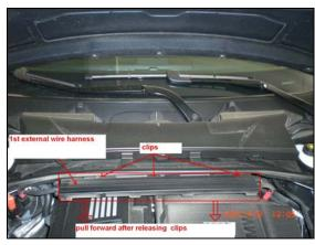
Step 3: Removal of center cowl cover 1<sup>st</sup> external wire harness
