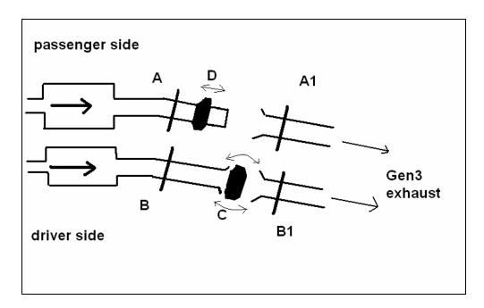
Adjustment of the exhaust can be changed by allowing sealing gasket ring "D" to move forward or backwards before tightening the flanges "A" to "A1" and "B" to "B1". This adjustment will allow for movement left to right and right to left for proper clearance at cross-member and trunk spare wheel well.
