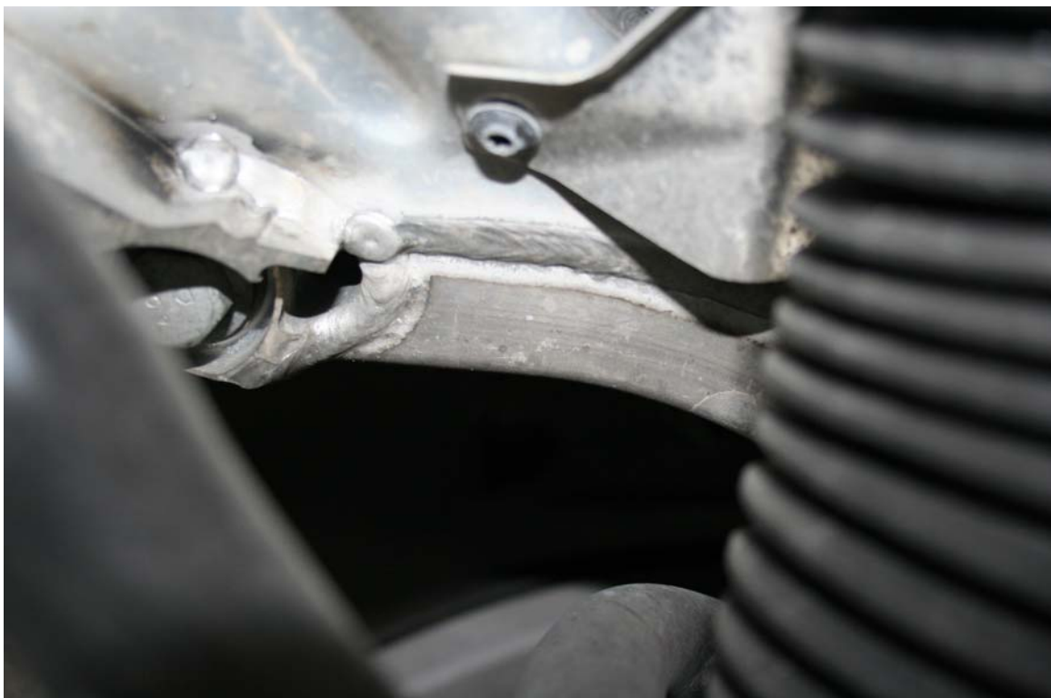
Power steering rack moved out of the way. Do not disconnect steering coupling, just let it hang down.
