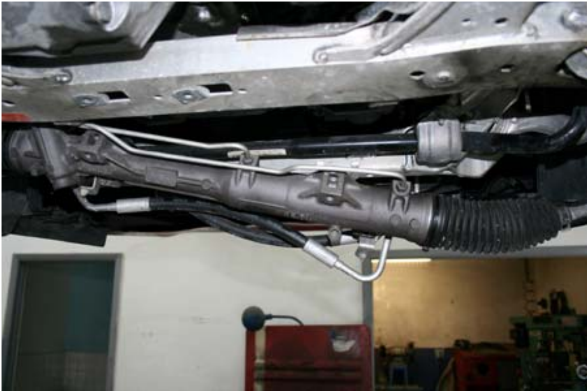
Power steering rack moved out of the way. Do not disconnect steering coupling, just let it hang down.
