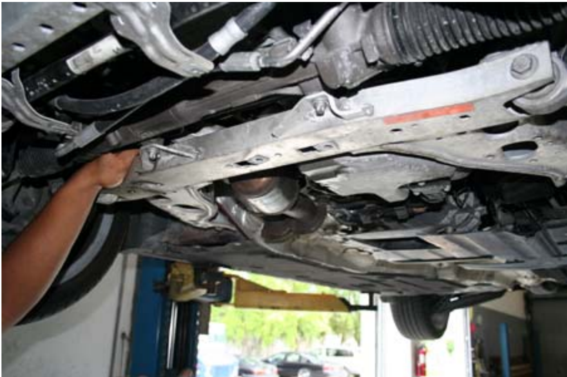
Remove both bolts holding the power steering rack on the subframe and pull it forward and down a little to make space to reach the downpipes(2 – E12 torx and 2 – 16mm nuts)
