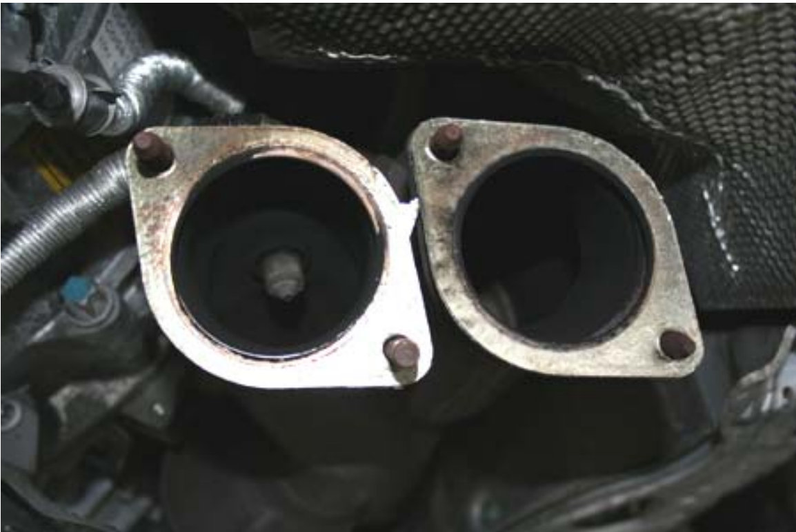
Downpipes with exhaust pulled back/down out of the way
