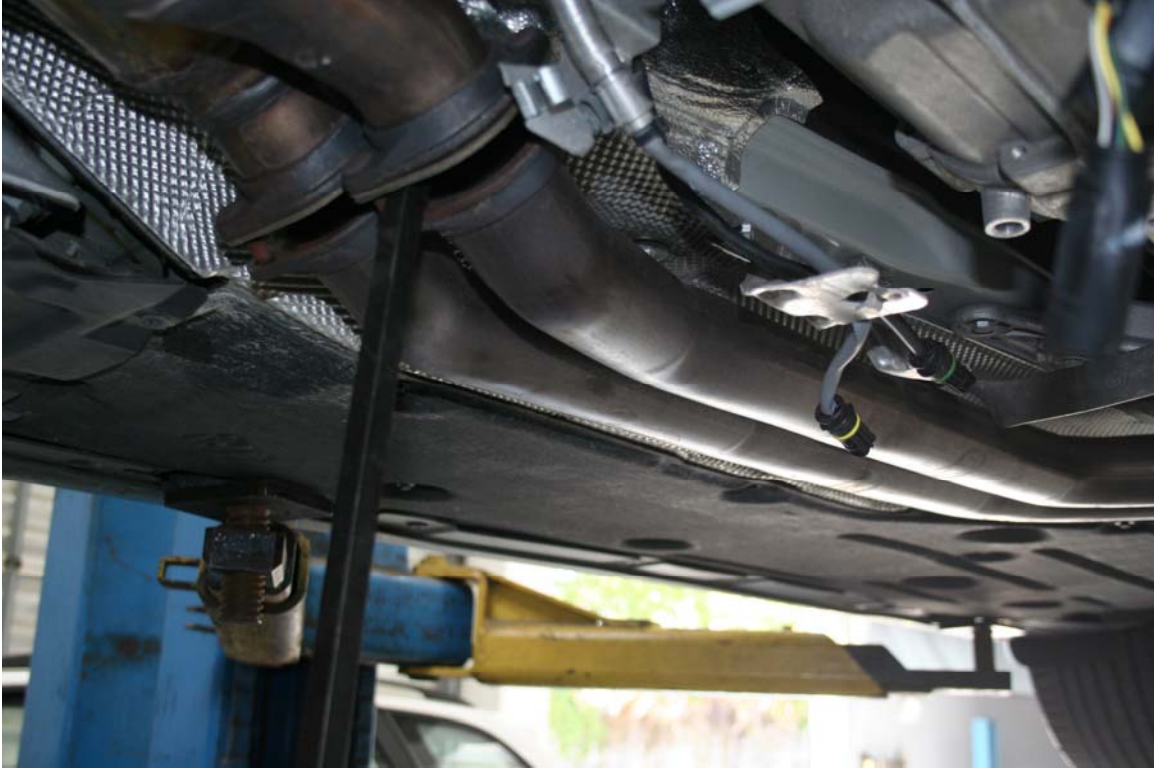
Pull/pry exhaust down and back until the downpipe bolts are free.
