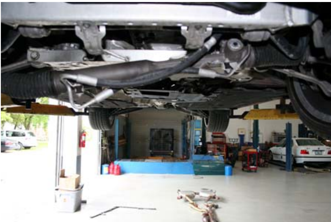
Pull power steering rack out of mounting holes and pull forward and down to make space.
