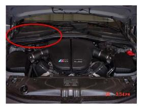
2. Lift where shown and slide the plastice brace out to the right
