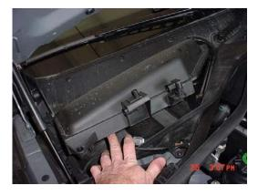
5. Next Release the 4 13mm Plastic Nuts and Remove the T20 Screw. Remove the entire assemble to access the electronic box
