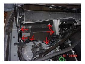
7. The DME is in the Back of the Box. Remove the two large black connectors by pulling the release tabs to the left and right
