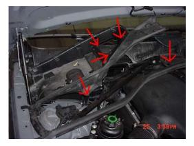
6. Loosen the 5 5mm Allen Head Screws and Slide the white triangle to the unlock position. Now remove the cover
