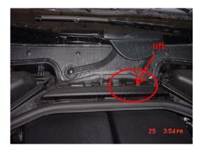
3. Next Pry down the Metal Bar, Disconnect the two electrical connectors and release the 13mm plastic nut
