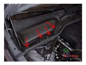
4. Lift up and Remove the filter Box
