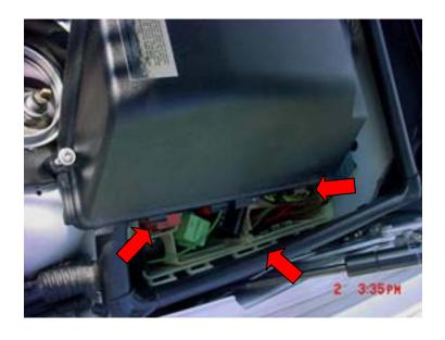
Continue removing ECU cover, the cover is hinged at the bottom.
