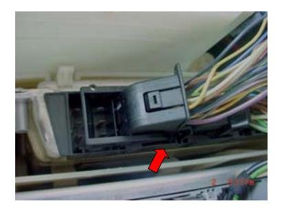
With slide lock out of the way, now pull connector up and out.
