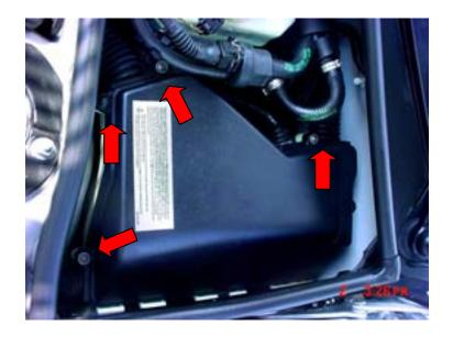
Unscrew cover using either a Torx T25 or a 5mm allen wrench.
