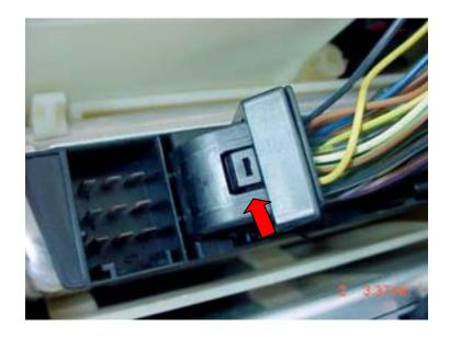
Push down on pin to release lock.
