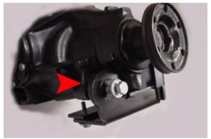
3. Mount the AA differential support bracket so that the circle ring is on top of the original circle hole that holds the rubber mounting and tap it gently so that it starts to sit on top of the circle, install the original differential bolt and catch now then thread it until snug.
