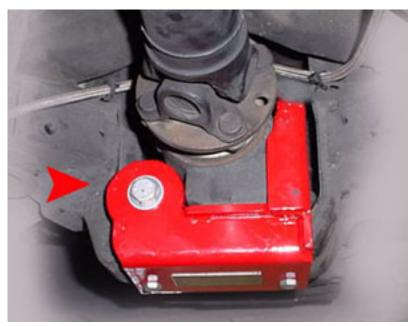
7. Now tighten the main differential bolt securely to at least 45-50 ft/lbs.
