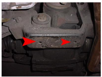
2. Take a 3/8" drill bit and drill through the (2) existing holes in the bottom of the carrier. These are the only 2 existing holes in the bottom of the carrier.
