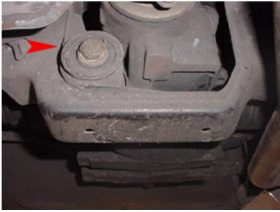
1. Take the stock differential front support bolt out and support the differential so that it does not go up or down. Use a jack or equivalent type of support.
