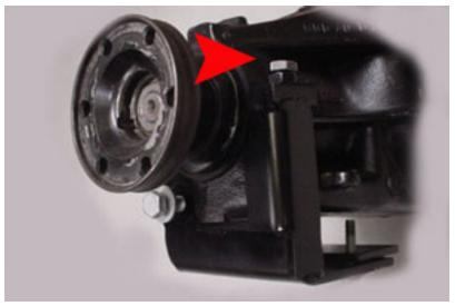
6. Take the pinch bolt (one with the 18mm head) on the AA DSB and tighten it approximately ¼-1/2 turns after it just touches the differential body. Tighten the lock nut to prevent the bolt from loosening.
