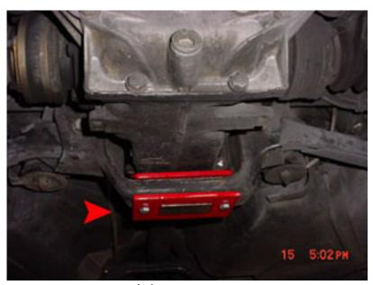
8. Tighten the (2) 8mm bolts at the bottom of the carrier to 18-20 ft/lbs. This concludes the installation.
