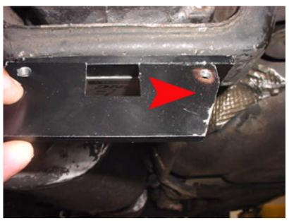
4. Install flat plate with beveled side facing passenger side (right side).
