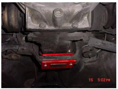
5. Slide the extra flat bracket supplied between the differential carrier and the differential so that the threads align with the holes in the AA DSB - Differential Support Bracket. Catch the supplied 8mm bolts using a 13mm socket and snug them down.
