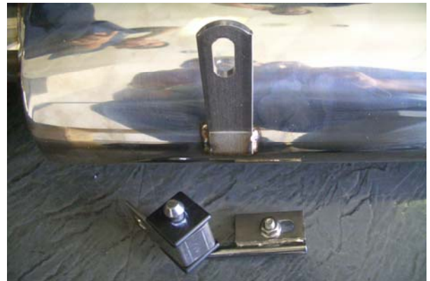
Installing the rear exhaust side brackets
