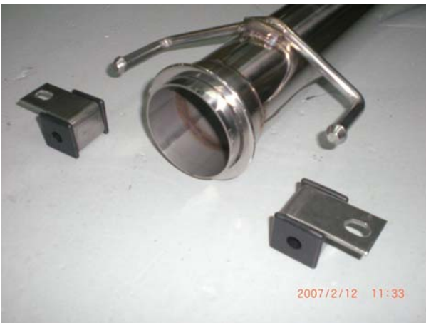
This is the MID SECTION with mounting tabs -Section with Tab ends faces the rear of the car -Tabs ends are to be on the TOP section of this pipe
