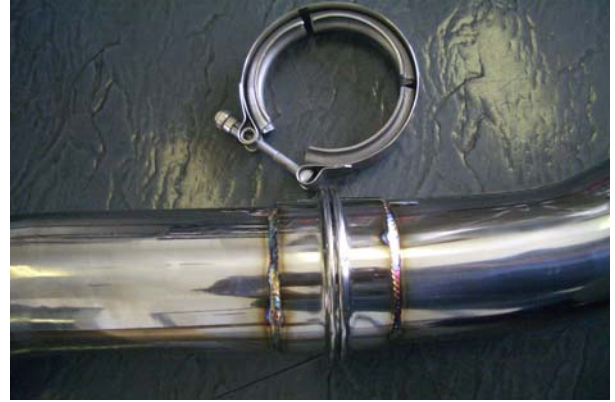
No gaskets required here. Only V-Band clamps are used
