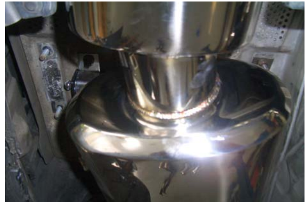
Driver's SIDE (LEFT Side) -Use the Long Bracket -Mount to inside of the muffler brace -Rubber mount bracket faces the rear of car
