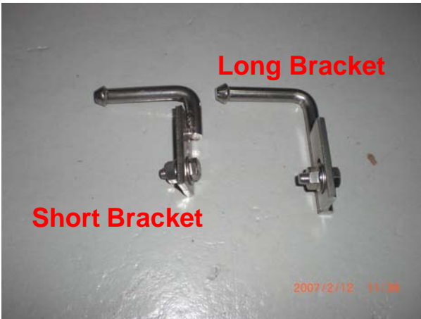
Installing the rear exhaust side brackets
