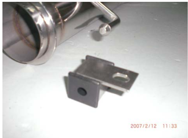
Each rubber mount has a FLAT plate on one side -FLAT plate must always be on top and resting against the car body
