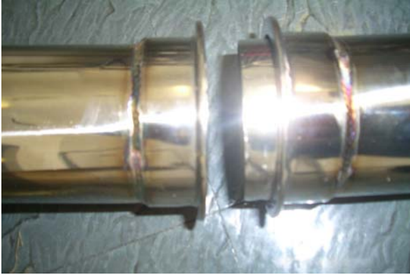
Each exhaust mounting section has a MALE and FEMALE end for a easier, more secure install
