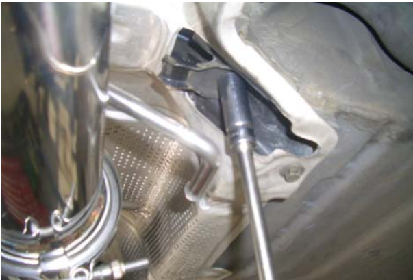
Remove existing Factory mounting hangers in the center body area -There will be one on each side of the driveshaft tunnel
