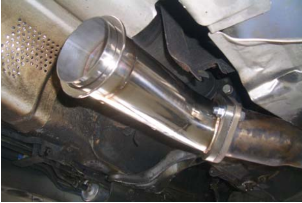
Mounting Front SHORT pipe with 3.0" exhaust gasket with bolts & nuts
