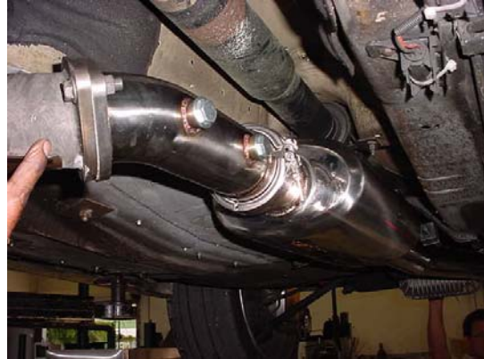
Mounting FRONT resonator or OPTIONAL straight thorough pipe with V-Band clamp to Front SHORT Pipe
