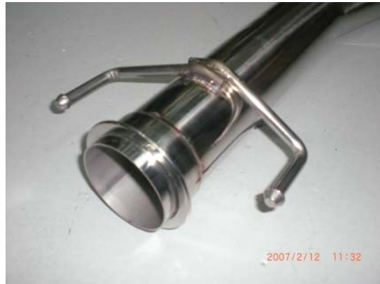
Mounting FRONT resonator to MID SECTION with mounting tabs
