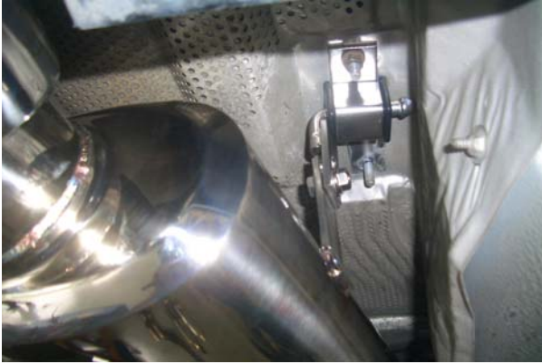
Passenger's SIDE -Use the SHORT BRACKET -Mount to outside of the muffler brace -Rubber mount bracket faces the rear of car
