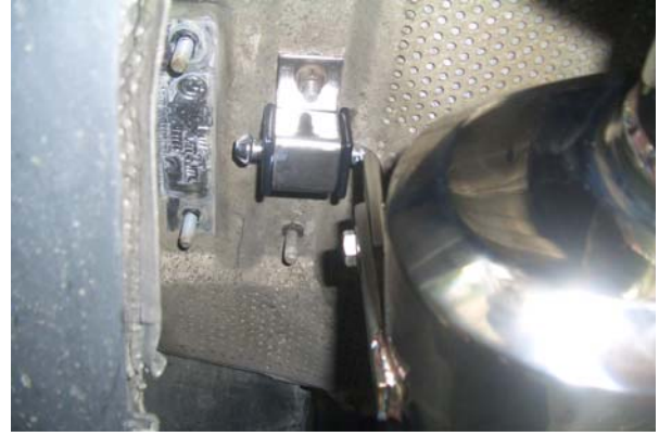
Driver's SIDE (LEFT Side) -Use the Long Bracket -Mount to inside of the muffler brace -Rubber mount bracket faces the rear of car
