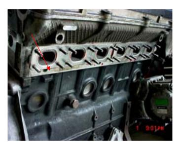
Removal of the factory exhaust manifolds using a 11mm socket.
