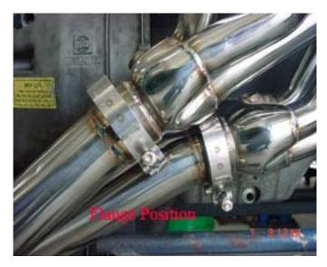
Install both 2.50" V band clamps to connect the Y pipe to both AA race headers.
