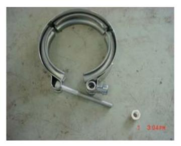
Before installing the Y-Pipe, the V-band clamps have to be opened first.
