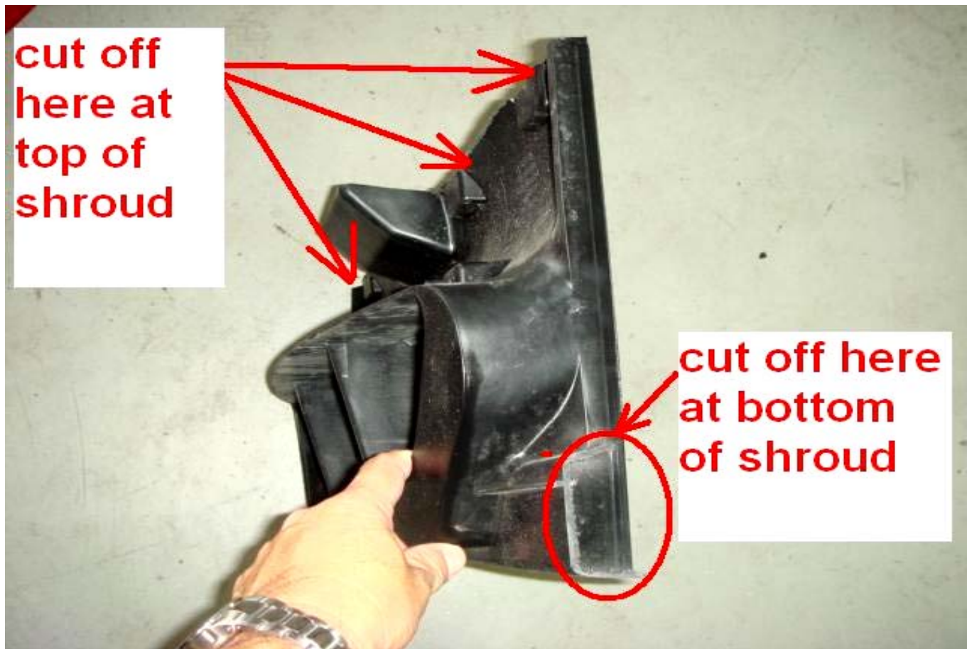
These are the areas to be cut. Hang down the bumper to get enough space to cut of the bottom half of the shroud.
