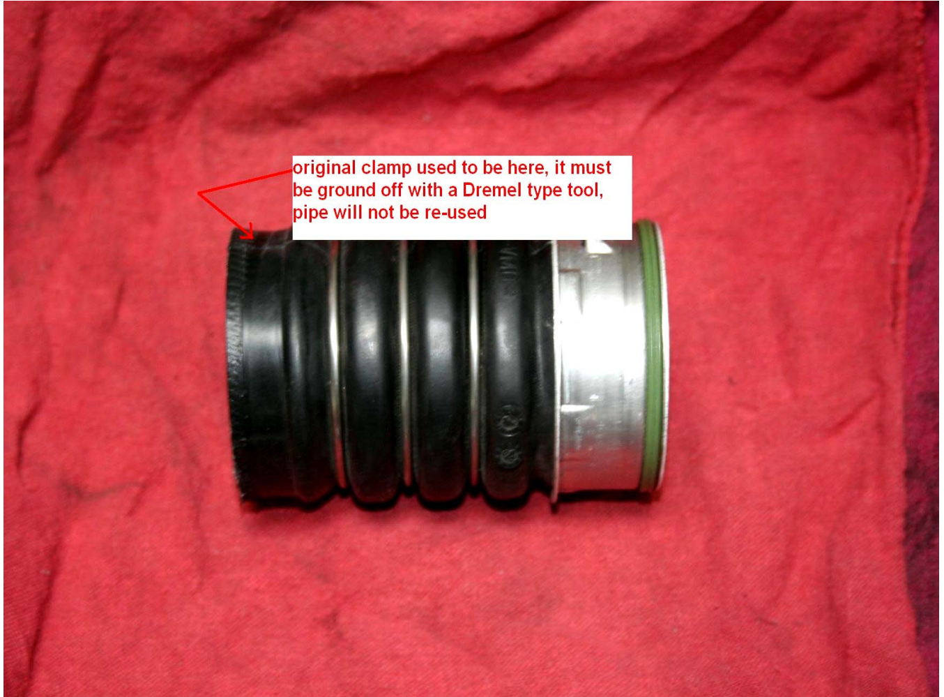
Right side pipe (passenger). New pipes will be supplied with the AA intercooler.
