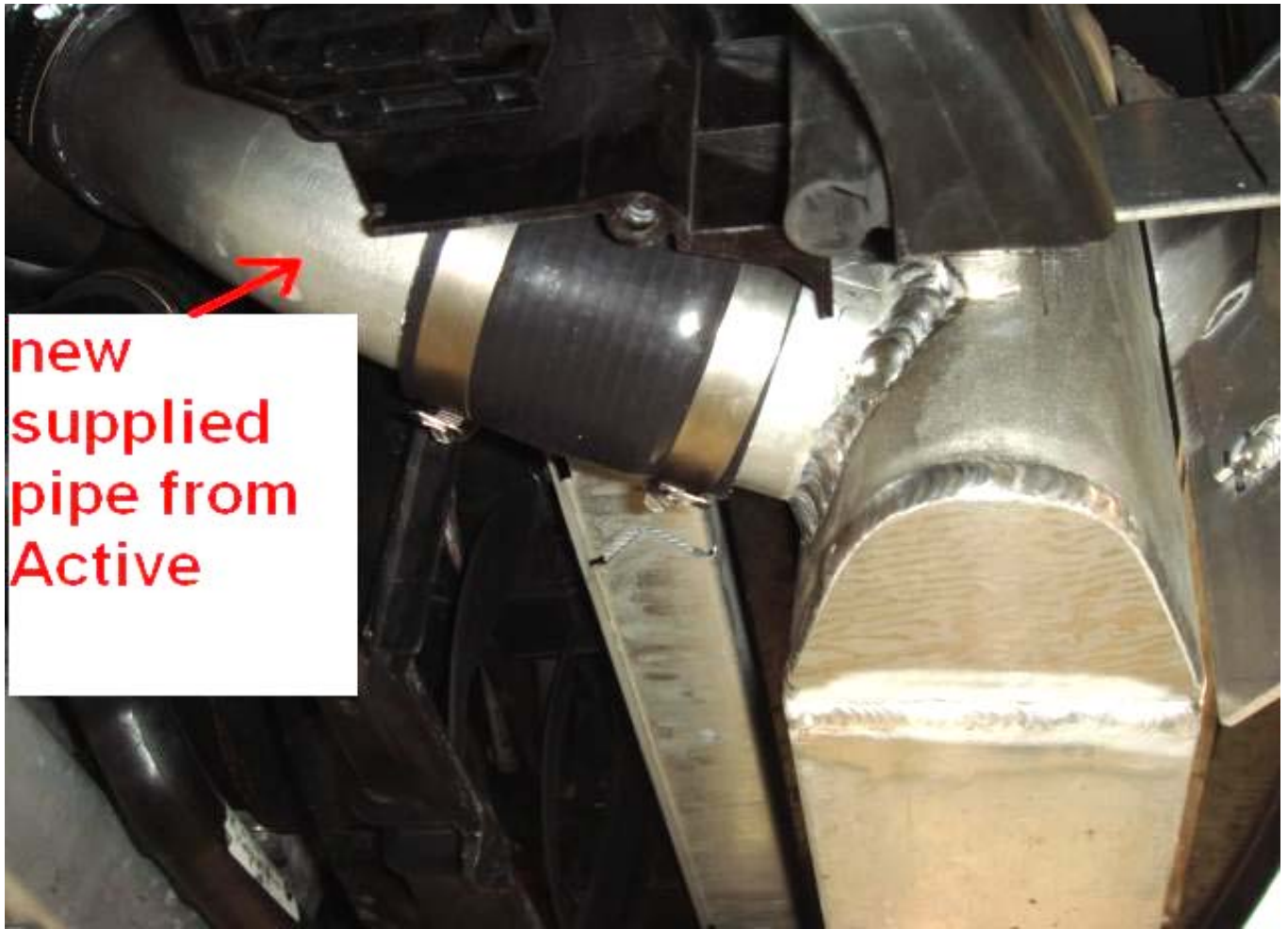
Attach passenger side pipe from turbo. Tighten all clamps.
