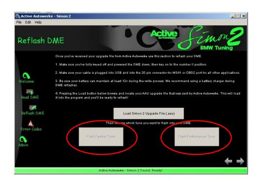
6. And .aau file will be send to you and that file will contain inside the tuned file and the original file , the one to the right Flash Performance tuned is the tuned file and the one to the left Flash Factory Tuned is the original. Flash the car via ODBII and remember to switch the ignition on and use a battery charger.
