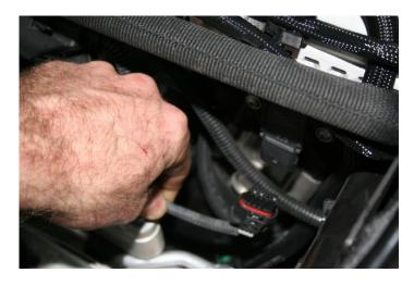
end of harness plug, reattach female end to original sensor wire.
