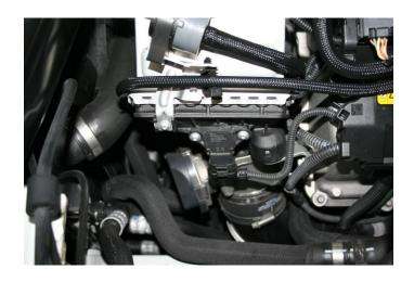
Unlock sensor plug (usually Grey locking tab) and replace with male
