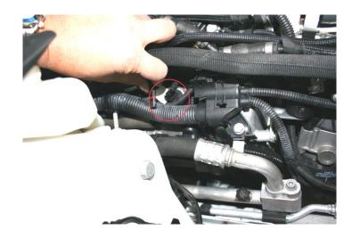
• Cam sensor ports at back of engine. (Early version)
