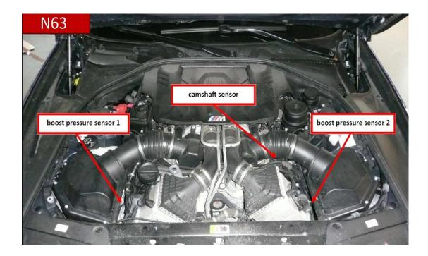
The Active 8 harness has 3 labeled connections: boost pressure sensor 1, boost pressure sensor 2 and the camshaft sensor. Note: Gen 2 harness include a (Red) power and (Black) ground wire. These can usually be routed towards battery lug in engine bay. Connect Red (fused) power to battery lug and ground to suitable chassis location. PICTURE ABOVE: late model cars. Cam sensor early model, located towards back by firewall (see picture below)
