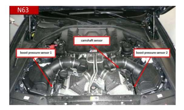
The Active 8 harness has 3 labeled connections: boost pressure sensor 1, boost pressure sensor 2 and the camshaft sensor.
