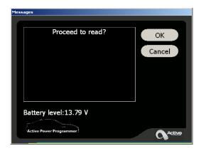
11. It will take up to 60 minutes to read the file out of the car. Make sure nobody disturbs the car during reading or writing to the ecu.
