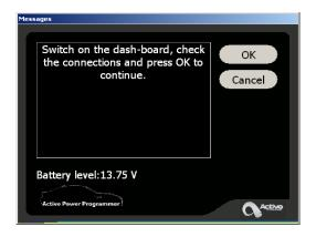
27. Next the Active Power Programmer will begin to program the new tuned file into the DME. This will take up to 60 minutes to complete. Please do not disturb the car while it is programming.
