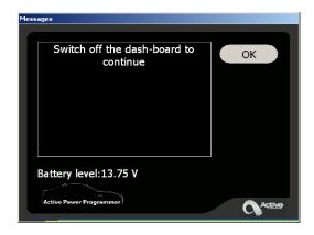
30. Now you can exit the Active Power Programmer software and remove the battery charger from the car. Now start the vehicle and verify that is running correctly. If you have any 'service engine soon', 'check engine' or 'transmission' error light. Use an appropriate scan tool to clear the errors. This is normal on most automatic or steptronic vehicles
