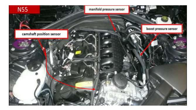
The Active 8 harness has 3 labeled connectors: Boost pressure sensor, manifold pressure sensor and the camshaft position sensor. On most applications the boost pressure sensor will be before the throttle (usually on the throttle body or throttle pipe) while the manifold sensor will come after somewhere on the manifold.
