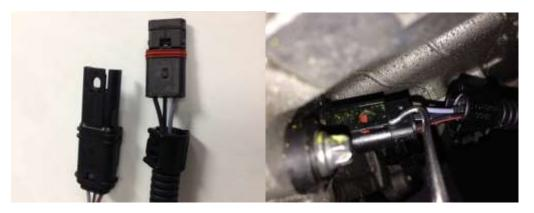
• Before attaching Active 8 module, connect Bypass Bridge and start car to make sure harness connections are good. Leave car off for 5 minutes before taking off bridge and attaching module.
