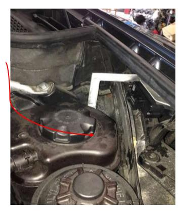
• Attach bracket using original coolant bottle 6mm bolt.
