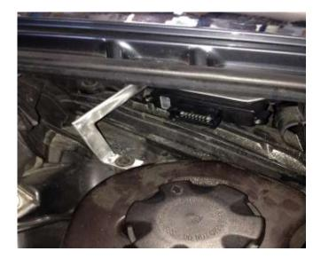
Tie strap harness in place and replace covers and air filter box.
