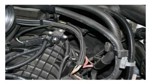
• Manifold pressure sensor connected to Active 8 harness.
