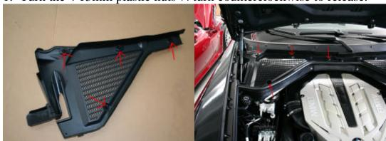
2. Now Turn the 3 13mm Plastic nuts to replace the panel. Also Unplug the electrical sensor
