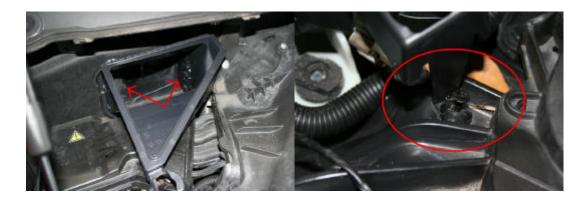
4. Now remove the electronic box cover by first releasing the spring clips. Then using a small screwdriver release the three retaining tabs
