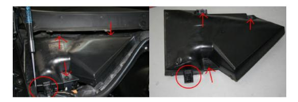
3. Release the two tabs inside the cowling. Then using a small flathead screwdriver, pry up on the inner pin to release the plastic rivet
