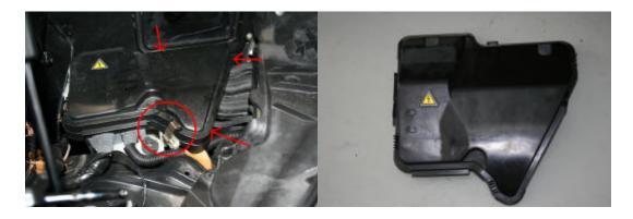
5. Now Remove the five electrical connectors from the DME and slide the unit up and out
