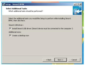
You need to plug the Simon 3 ODBII interface to the laptop and click next to install the proper usb drivers.
