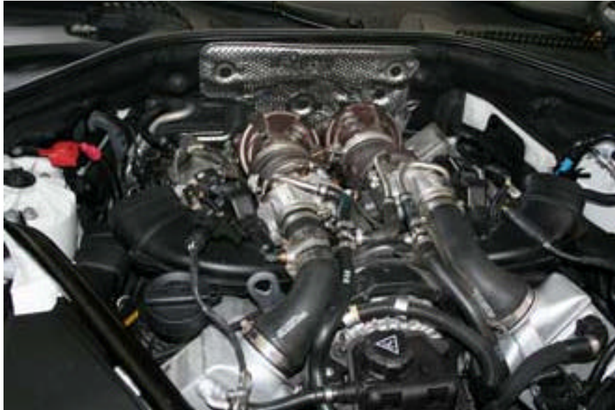
Step 64: Release turbo V-BAND clamps to down pipes
