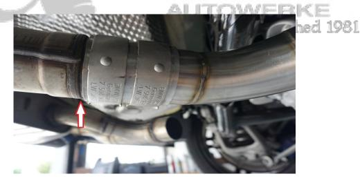
Slide both clamps over the exhaust pipes until the clamps are about halfway over both ends of the pipes. Then proceed to tighten all clamps. See image above for example.
