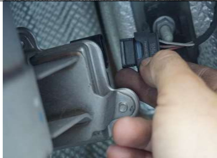
4. DISCONNECT EXHAUST FLAP MOTOR WIRES.
