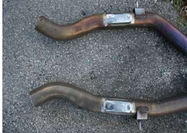
3. MID PIPE AFTER CUT.
