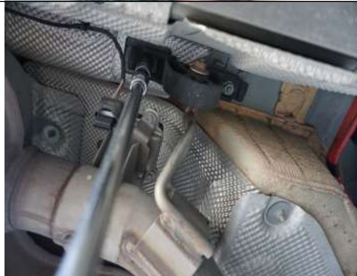
5. REMOVE BOTH EXHAUST MOUNTS WITH 8MM SOCKET.
