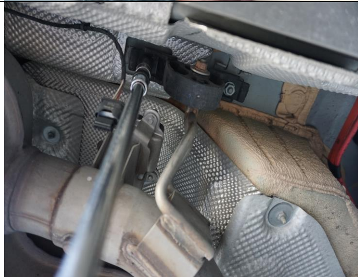
5. REMOVE BOTH EXHAUST MOUNTS WITH 8MM SOCKET.
