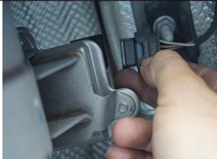
4. DISCONNECT EXHAUST FLAP MOTOR WIRES.
