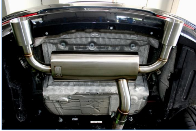
Under carriage view of exhaust installed.
