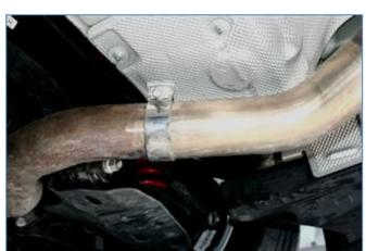
Position muffler and tighten clamps.
