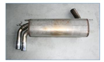
To remove factory exhaust the pipe will have to be cut.
