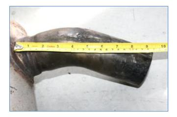
Measure 9.5 inches from back of the muffler pan and mark. (Bottom of pipe)
