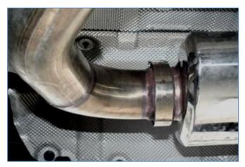
Leave clamps loose and slide muffler pipe unto factory pipe.
