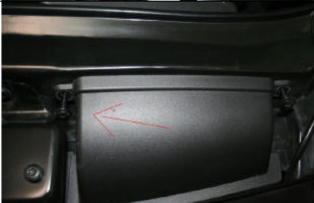
Screws to remove air duct.
