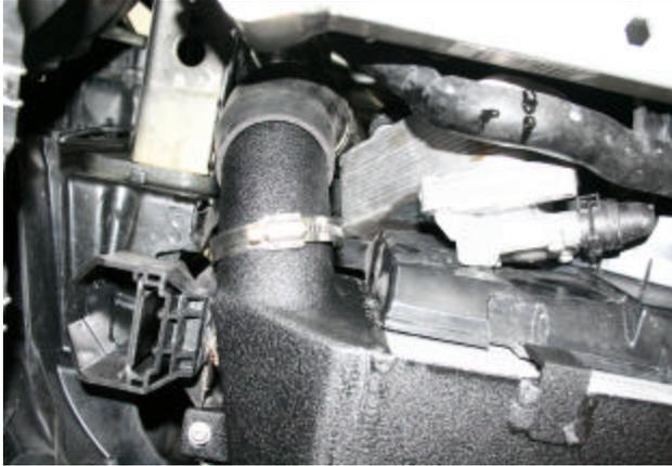
Inter cooler will fit around Automatic transmission cooler
