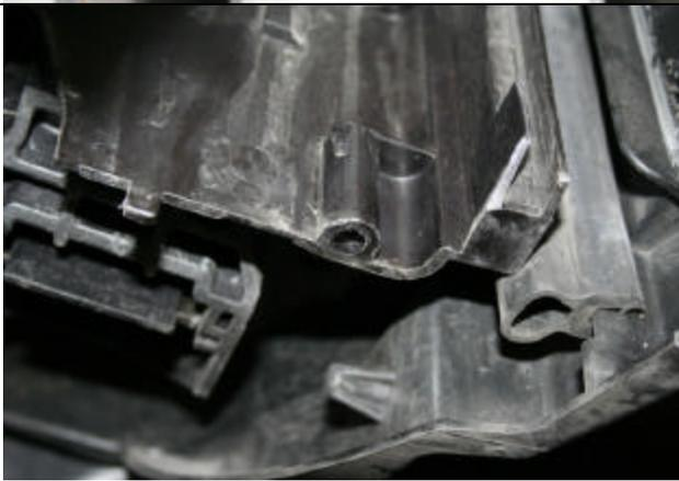
Use back original mounting holes and screws for AA inter cooler.
