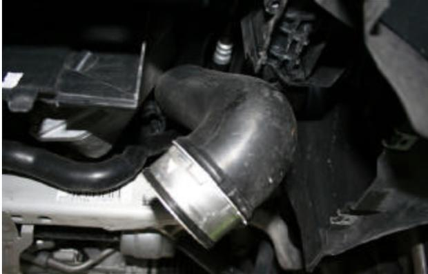
Turn and pull out pipe from under the car.
