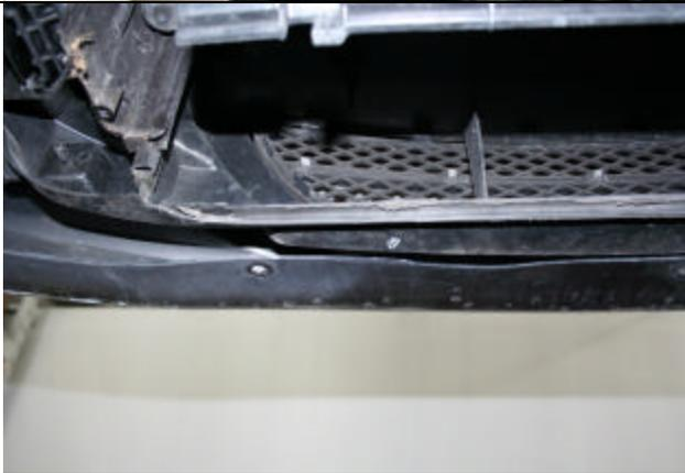
Cut 1 inch off of the forward lip so that inter cooler will be able to pass into space
