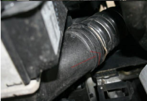
Pull clips for pipes on both sides
