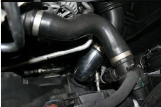
Feed new AA pipe through the top and adjust.
