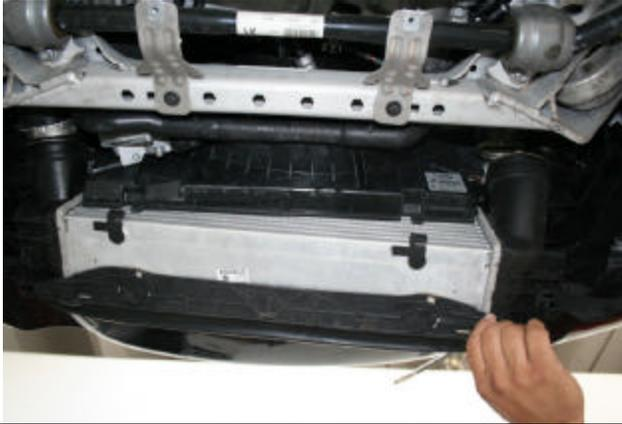
Pull down on inter cooler, stretching spoiler to let inter cooler pass.
