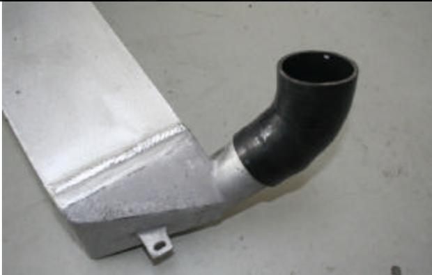
Pre-set 45 degree 2.5 inch Silicone hose on drivers side (left) of the inter cooler.
