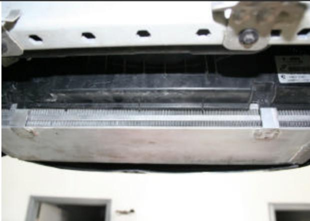
Align hoses with pipes and radiator shroud with tabs.
