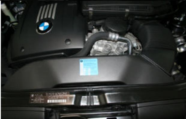
Remove air duct. This will give you more space to adjust the new pipe.
