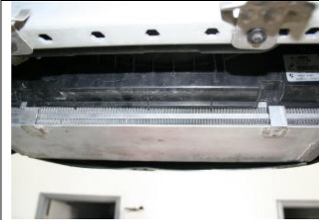
Fit new inter cooler with hoses in to opening by stretching spoiler lip.
