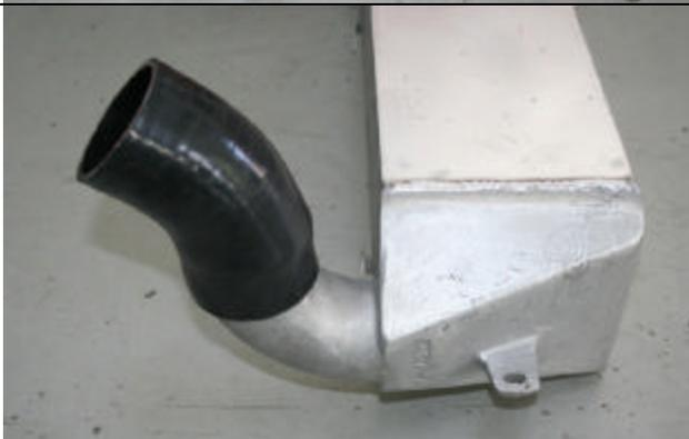
Pre-set 45 degree 2.5 inch Silicone hose on the passenger side (Right) of the inter cooler.
