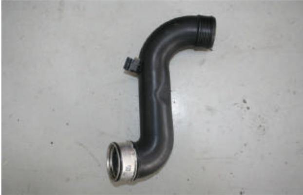
Note tab on side of pipe; pull up on pipe from the top to release the tab from the radiator.
