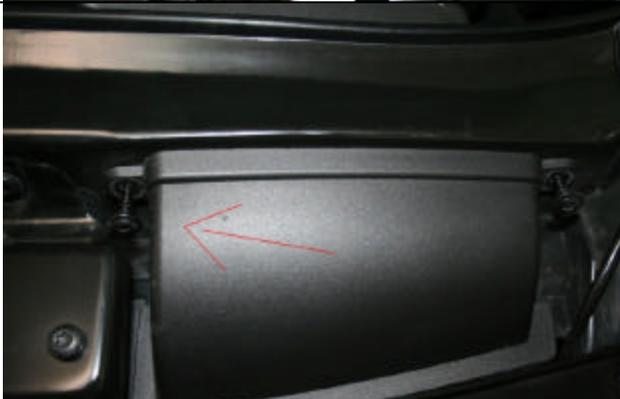
Screws to remove air duct.
