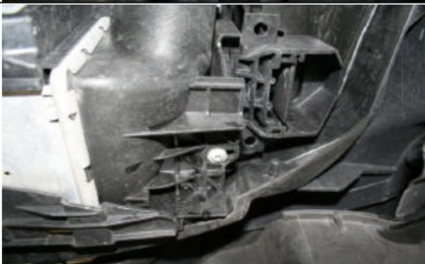
Remove T25 Torq screws from both sides of inter cooler
