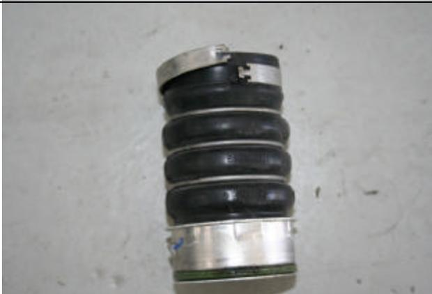
On passenger side of car (Right) locate where clamp is joined and use long screw driver to pry apart. Remove flex hose.
