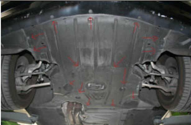
Remove under panel (8mm head screws)
