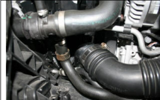
Position pipe so that it is not touching anything. Tighten clamp to keep hose in position.
