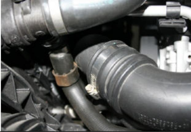
From the top of the car driver's side (left) loosen discharge pipe clamp (8mm).
