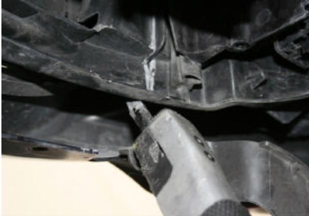
Cut carefully with Air saw
