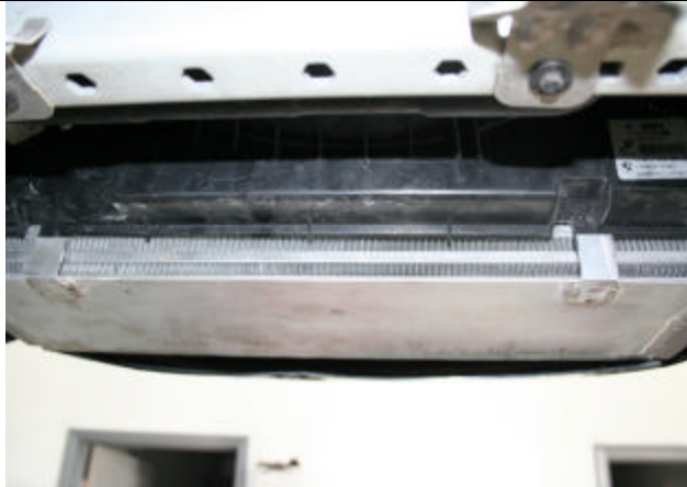
Align hoses with pipes and radiator shroud with tabs. Remove inter cooler and set clamps.
