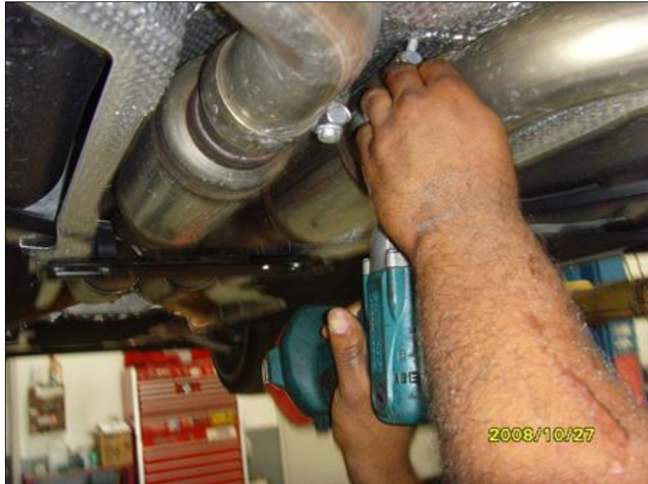
Disconnect rear muffler clamp
