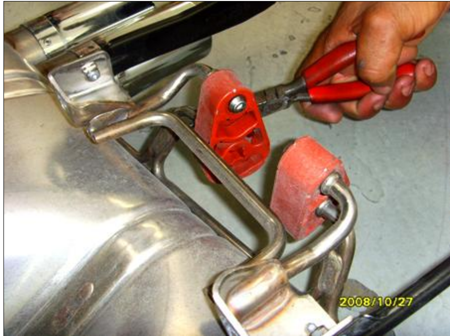
Using a needle nose pliers, pry away the RED rubbers from the factory muffler
