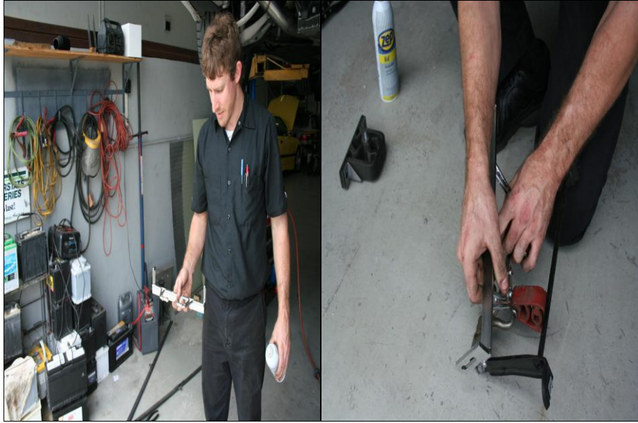
Transfer existing rubber mounts to new SPORT center bar.
