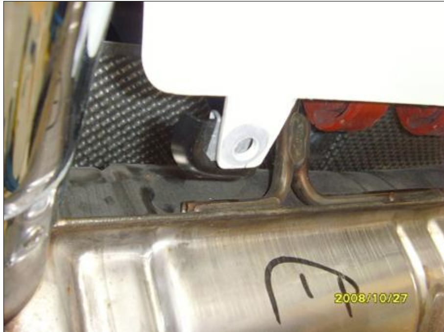
Disconnect rear valance from rear muffler support using a 8mm socket
