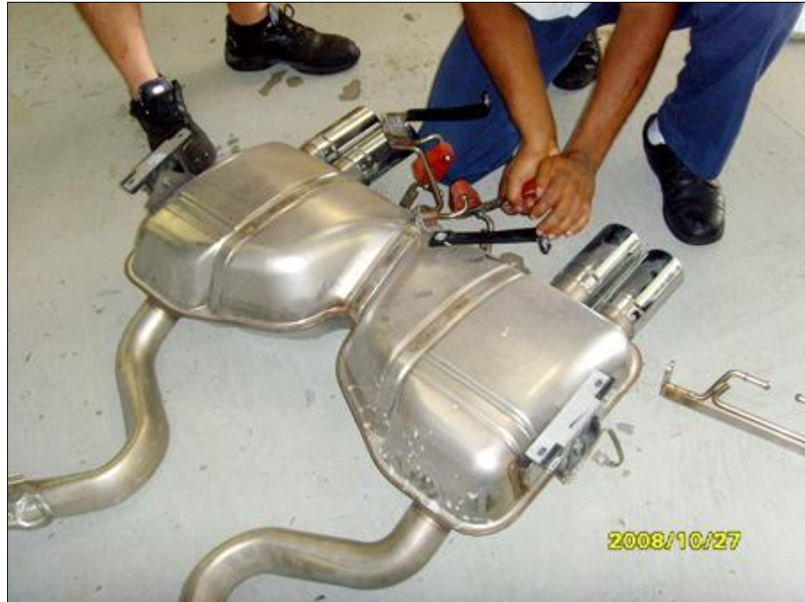
Removing away from the factory muffler
