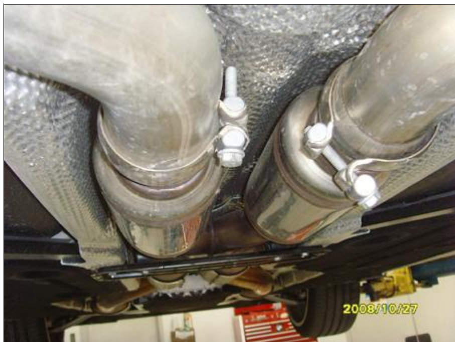
Disconnecting rear muffler clamp
