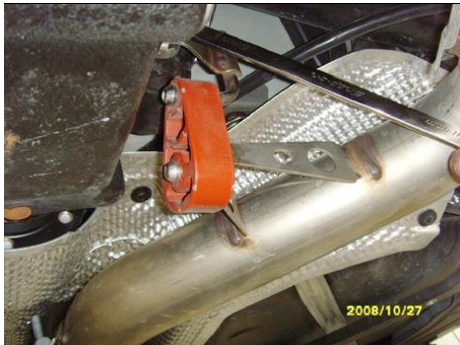
Disconnect exhaust hanger from body
