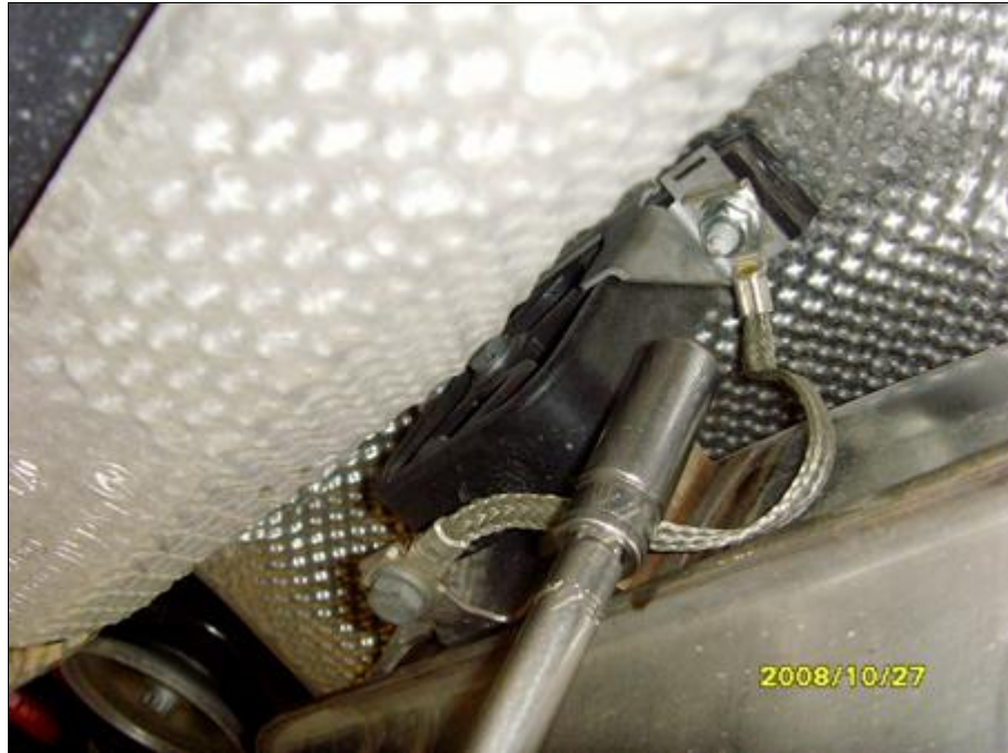
Disconnecting rear hanger on right side Ground strap will not be reused
