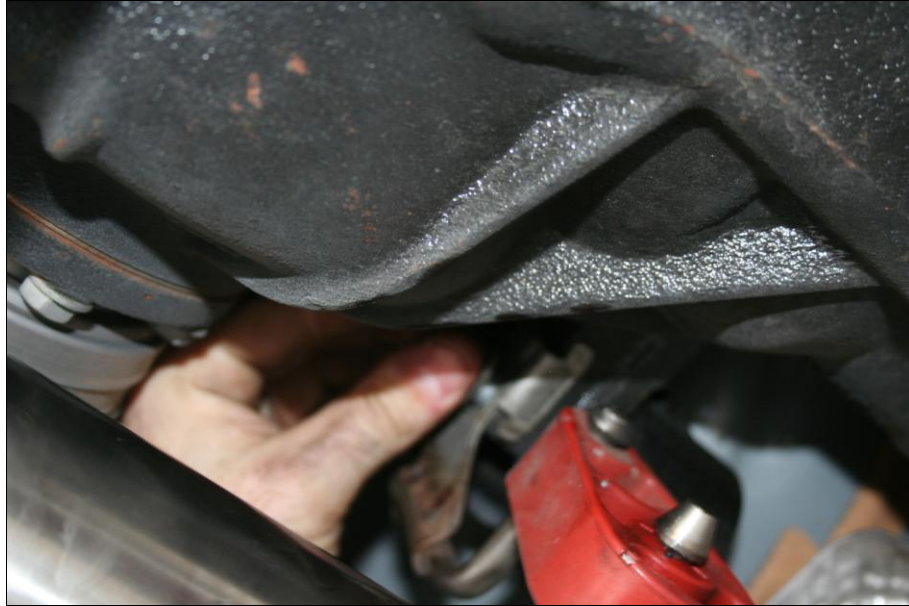
Mount hanger bracket to existing factory location.
