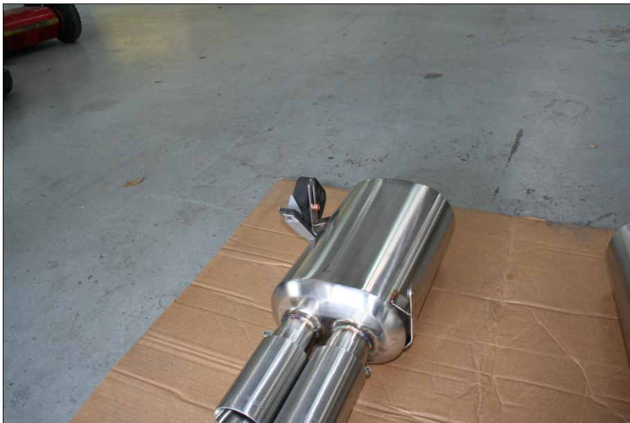
Transfer and install right (passenger side) exhaust hanger
