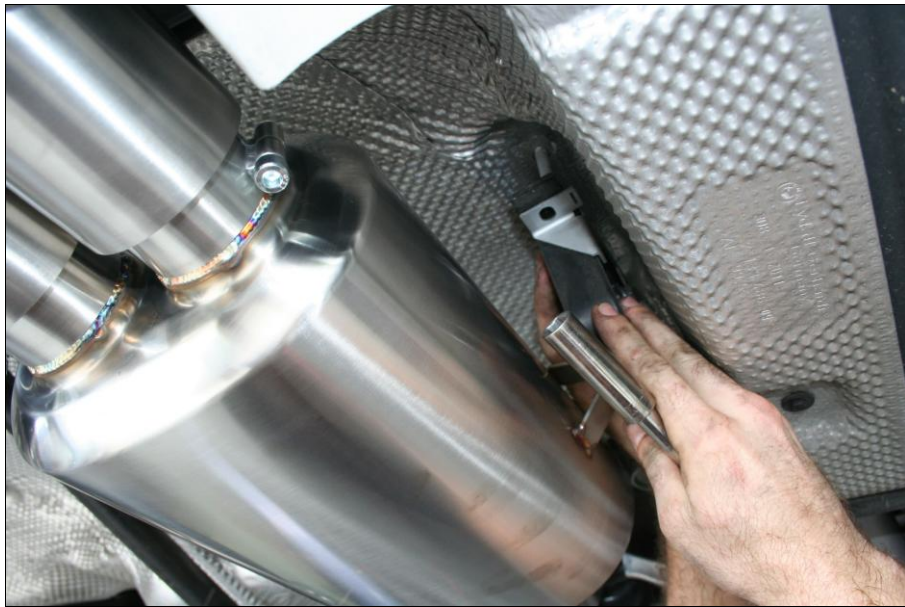
Install the side exhaust mount
