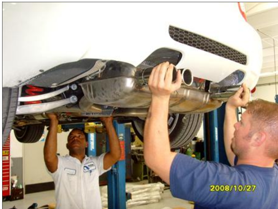
With the help of a friend, start to remove the factory rear muffler. Watch for interference from the rear valance while removing
