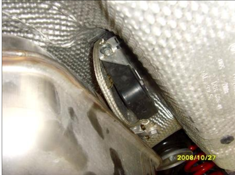
Disconnecting rear hanger on left side Ground strap will not be reused
