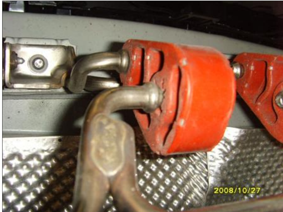
Disconnect rear center bracket from body. Assembly will be removed with the factory muffler
