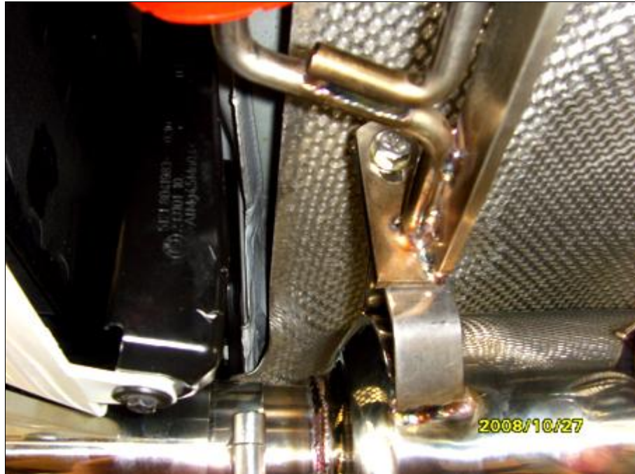
Connect the left rear Active Autowerke muffler to the center exhaust bracket
