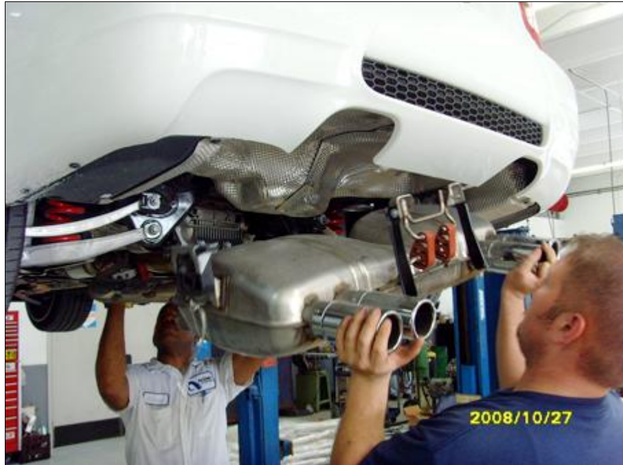
Factory rear muffler being removed with center bracket still attached
