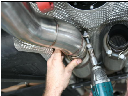
Tighten the front pipe clamps
