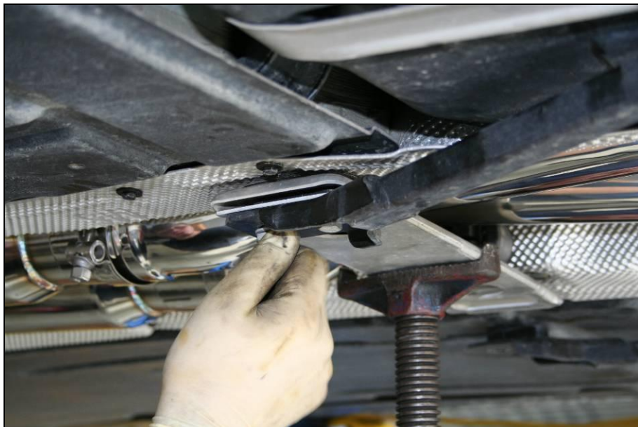
X-PIPE Cross member being installed
