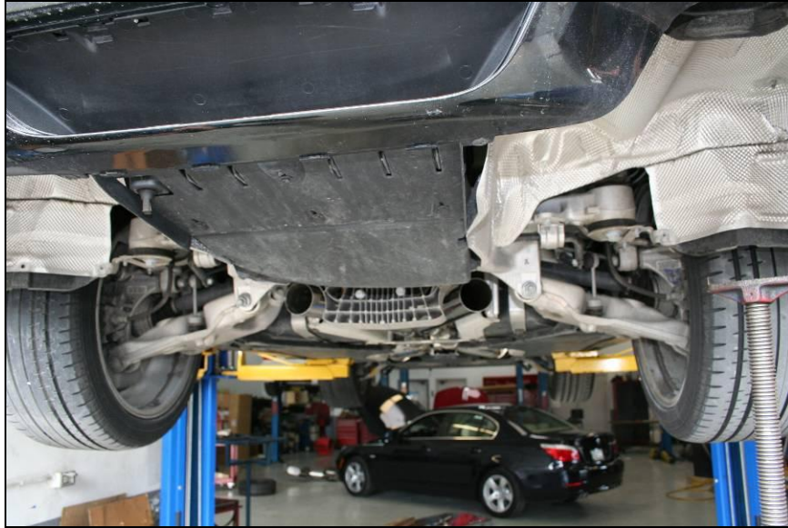
X-PIPE exiting around differential. Waiting to be connected to rear mufflers.
