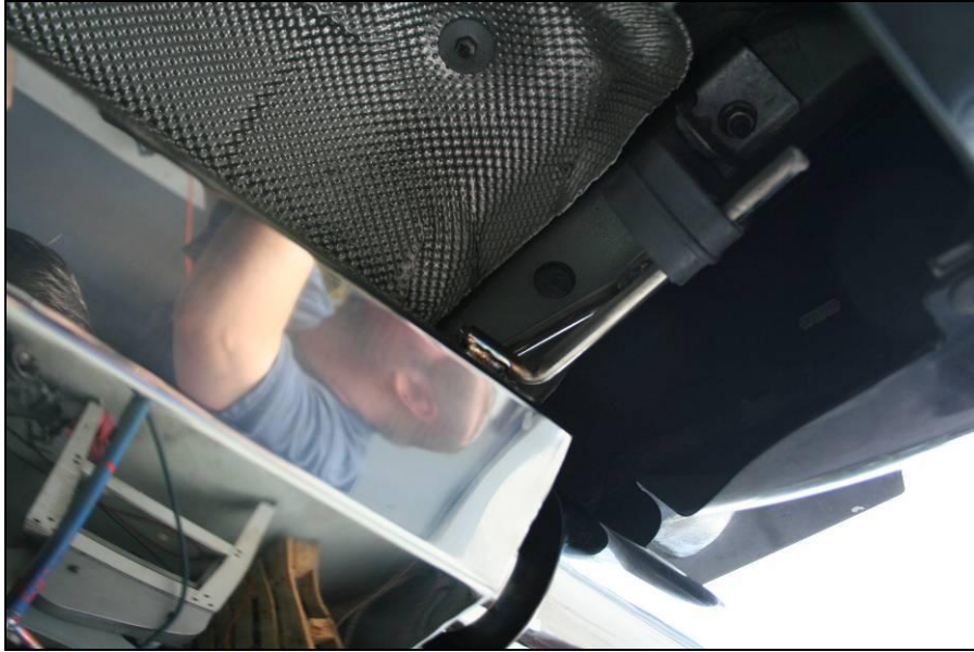
Rear mount on exhaust can installed to body rubber mount.
