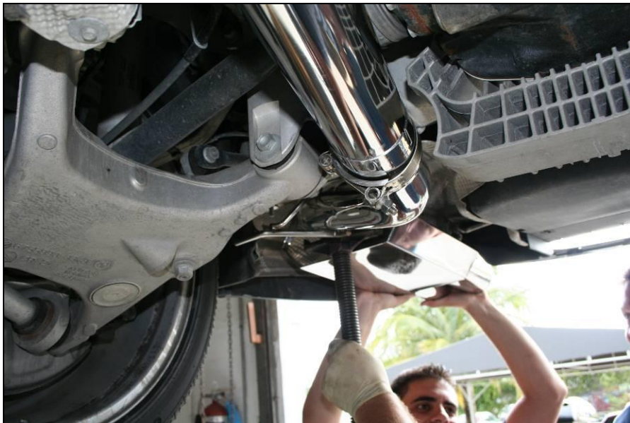
Support exhaust rear can while catching rear support mount.
