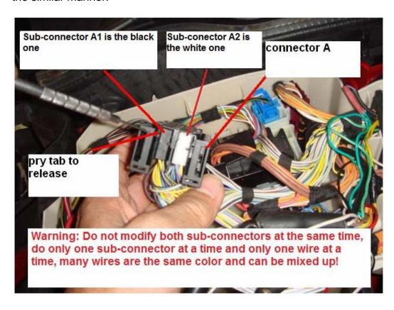
Take A1 and locate the slot numbers in the connector, they are numbered from 1-22 on one side and 23-44 on the other side. It is very important to locate the correct number slot before removing the wire, use the diagram below to assist you. Use the supplied heat shrink tubing to insulate the connection between the OEM wires and the AP2 connecting wires.
