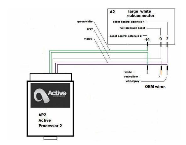
Re-install sub connectors A1 and A2 back into the connector A, tidy up the wires and use the supplied zip ties to tie wires neatly in place.
