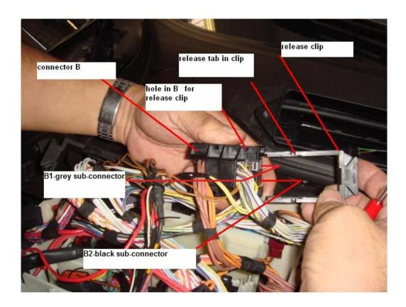
Take B1 and locate the slot numbers in the connector, they are numbered from 1-13 on one side and 14-26 on the other side. It is very important to locate the correct number slot before removing the wire, use the diagram below to assist you. Use the supplied heat shrink tubing to insulate the connection between the OEM wires and the AP2 connecting wires.
