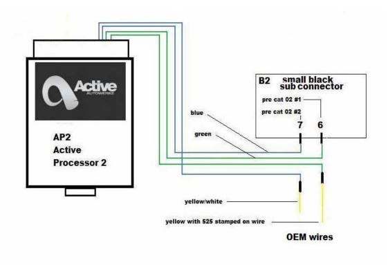
Re-install sub connectors B1 and B2 back into the connector B, tidy up the wires and use the supplied zip ties to tie wires neatly in place.
