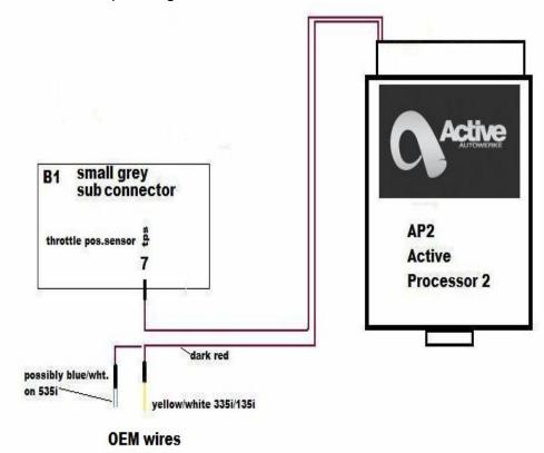
Take B2 and locate the slot numbers in the connector, they are numbered from 1-13 on one side and 14-26 on the other side. It is very important to locate the correct number slot before removing the wire, use the diagram below to assist you. Use the supplied heat shrink tubing to insulate the connection between the OEM wires and the AP2 connecting wires.
