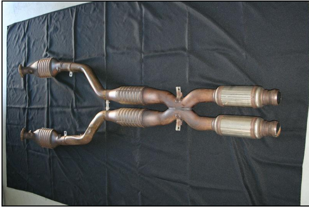
Factory exhaust removed
