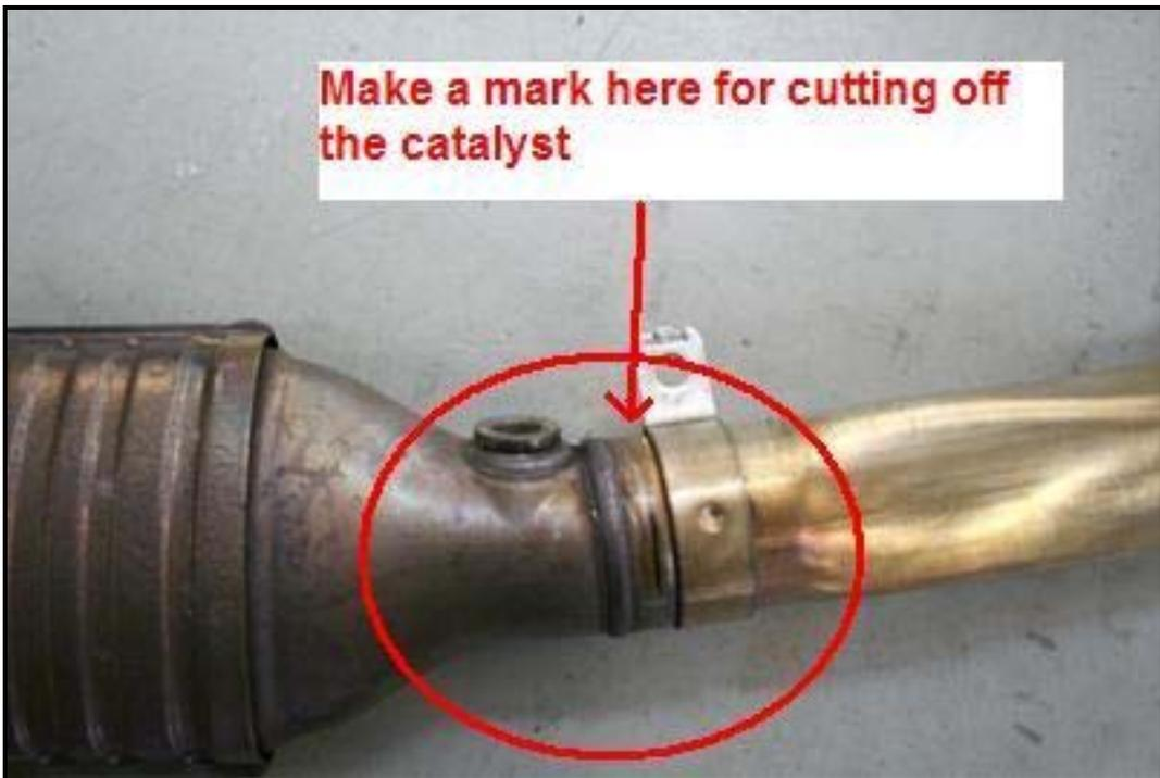
On the LEFT catalyst, there is a weld mark made by the factory. Approximately 10mm after the weld, there is a depression. Using a felt tip marker, make a mark all-around as a guide mark.
