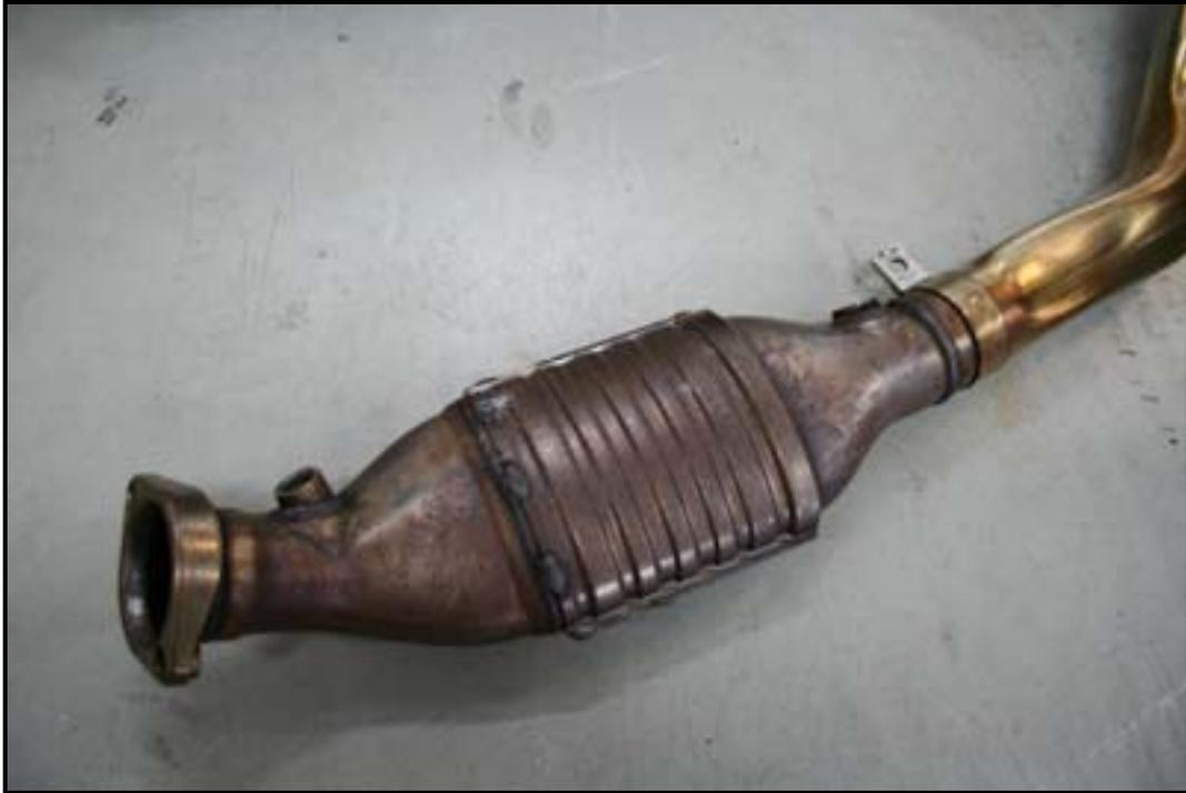
Picture of the LEFT side catalyst and the mark to be made for cutting off the catalyst
