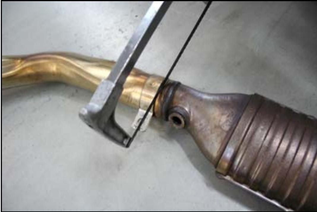
Using a hack-saw, cut off the LEFT catalyst
