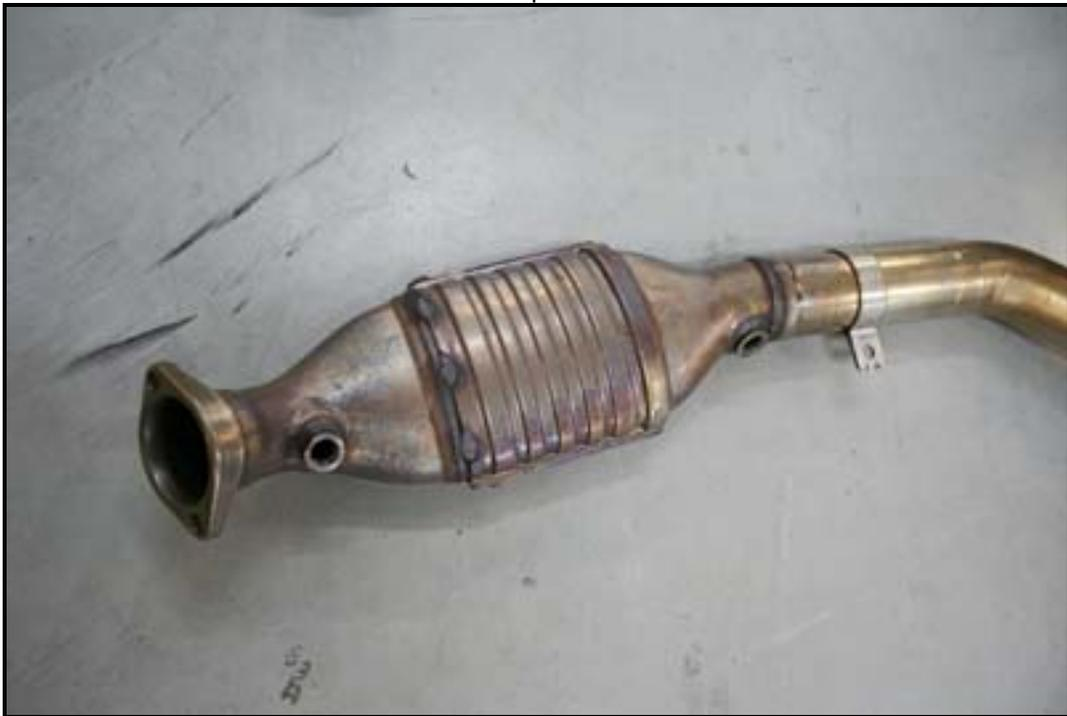
Picture of the RIGHT side catalyst and the mark to be made for cutting off the catalyst
