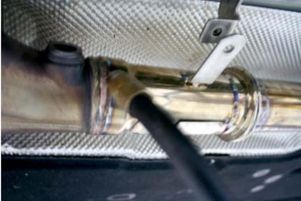
Position the STUBBIE between the factory catalyst and the Active X-PIPE and secure with the V-BAND clamp and other mounting hardware. The Stubbies have a sleeve making the pipes slide on for a partial fit.
