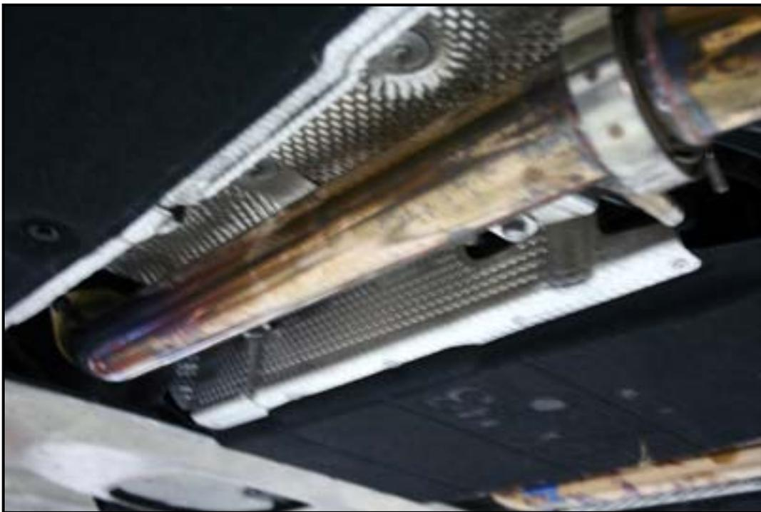
Remove the front pipes of the X-PIPE and install the cut off factory catalyst.
