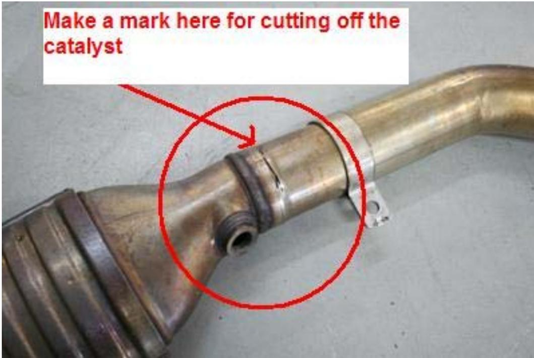
On the RIGHT catalyst, there is a weld mark made by the factory. Approximately 15mm after the weld, there is a depression. Using a felt tip marker, make a mark all-around as a guide mark.
