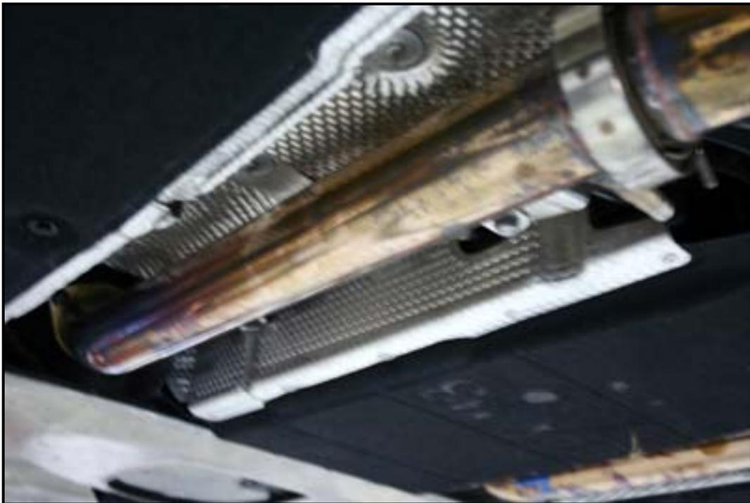
FRONT section of the Active Autowerke X-PIPE installed for race prep
