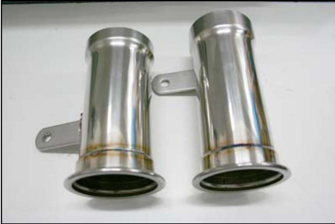
Set of Active Autowerke exhaust Stubbies for BMW E9X M3. Stubbies are of different heights, the taller one goes on the drivers (LEFT) side, while the shorter one goes on the passenger (RIGHT) side.
