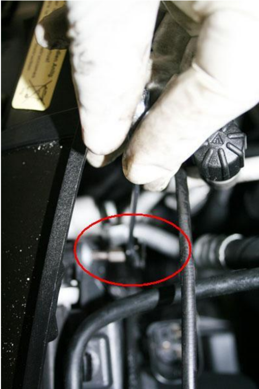
Remove bolt using Torx socket
