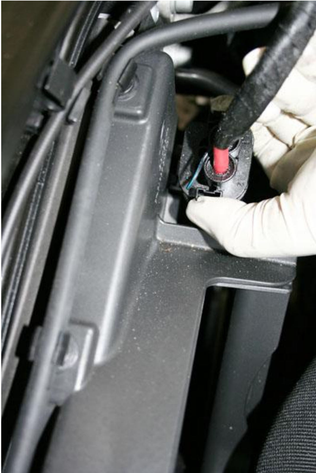
Disconnect engine aux fan connector
