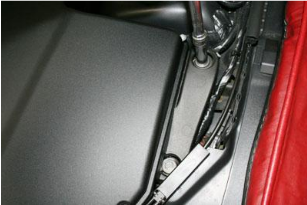
Unbolt using 10mm socket
