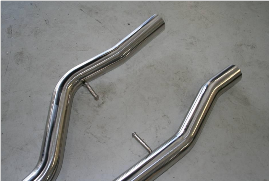
When mounting "X PIPE" make sure that mounting tabs faces down
