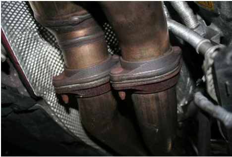
Separate the factory exhaust from the down pipes Remove entire exhaust system
