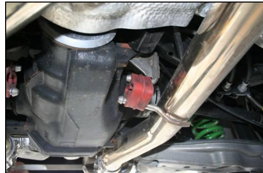
Mount "X PIPE" tabs to rubber mounts located around differential
