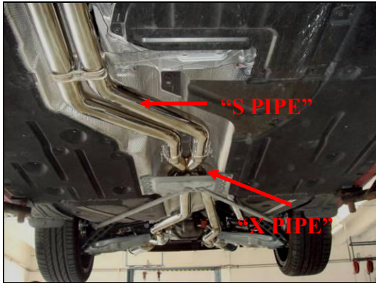
"X PIPE" mounted to "S PIPE"
