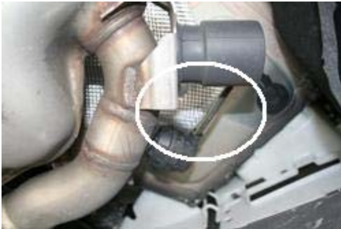
Driver side exhaust with vac line attached. Remove vac line connecting to vac actuator and plug with the screw provided. line
