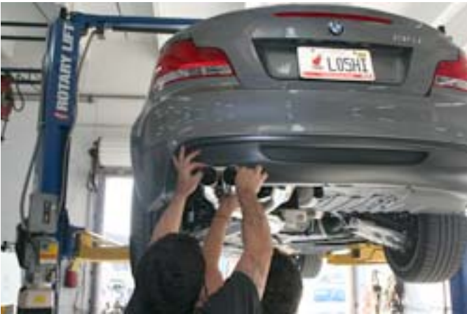
Adjusting the Active exhaust tip clearances. There are infinite adjustments with the use of the slotted brackets
