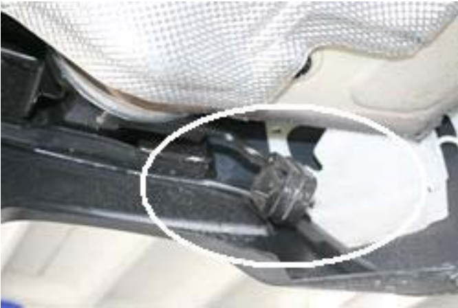
Driver's side hanger on the factory exhaust
