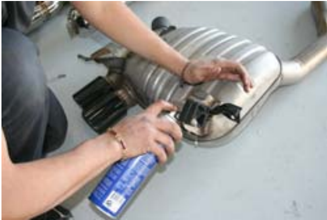
Using WD-40, spray the rubber to help slide off
