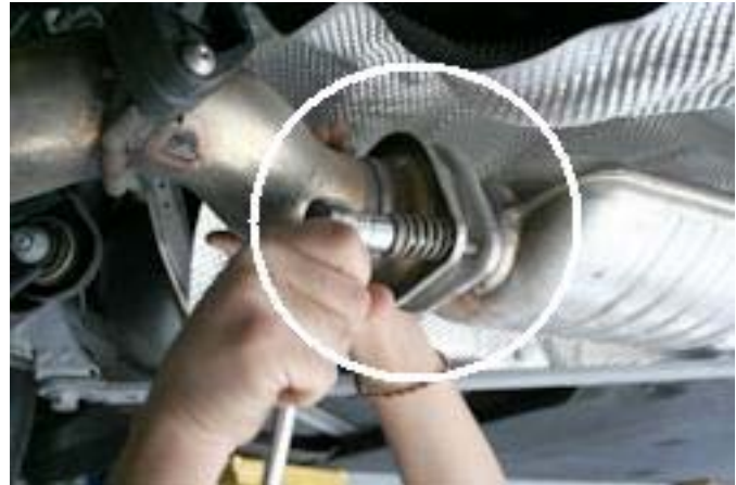
Tuck plugged vac line away. Use the heat shield to hide the vac
