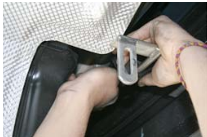
Mount Passenger side exhaust hanger. Then slide in the Active RIGHT exhaust mounting bracket
