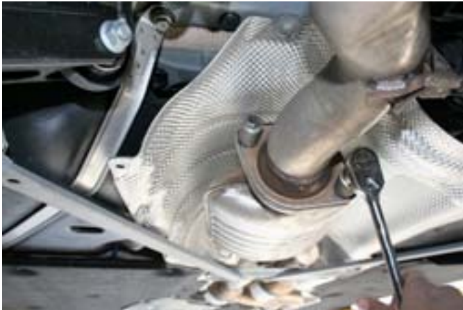
Use a 14m socket to remove the bolt with torsion spring.
