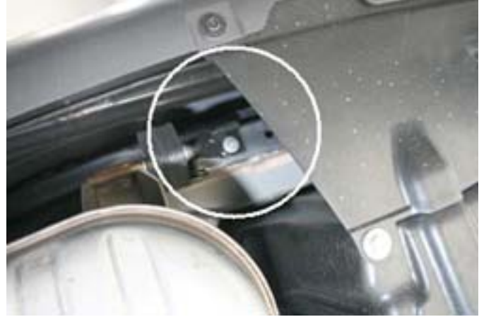
Passenger side of the exhaust. Remove using Torx E10
