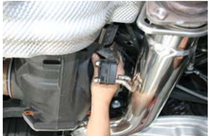
Connect the FRONT exhaust hanger
