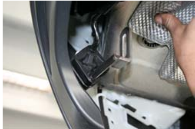
Install the Active LEFT exhaust bracket into the rubber hanger on the car
