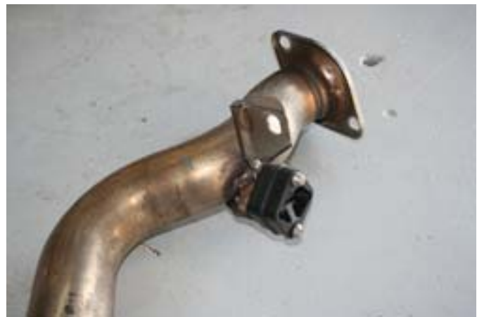
Front hanger on factory exhaust
