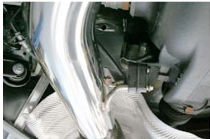
Connect the FRONT exhaust hanger
