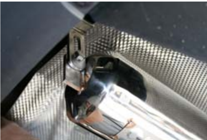
Use a washer with each bolt
