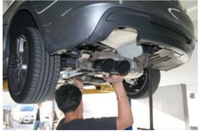
Removing the factory exhaust
