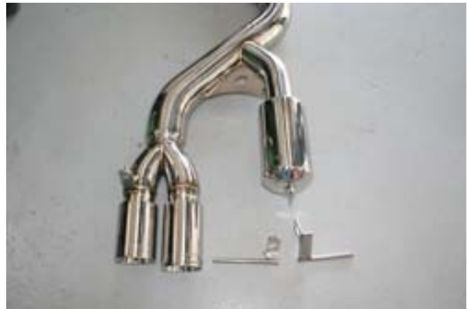
Active exhaust package ready for installation
