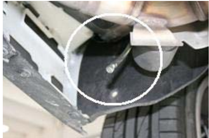
Tuck plugged vac line away. Use the heat shield to hide the vac
