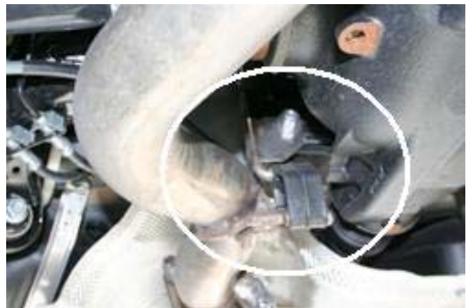
Remove the nut using a 18mm wrench
