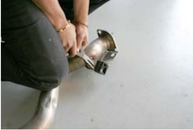
Using a pliers, start prying off the FRONT exhaust rubber then transfer to the Active exhaust
