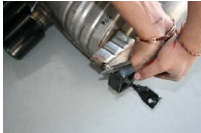
Use a pliers to help slide off the exhaust rubber
