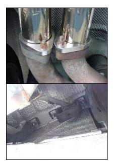
Remove the pipe connections where the pipes go into the stock rear muffler.
