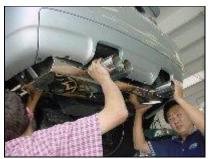
Lower the exhaust and push it towards the rear allowing the exhaust pipes to come loose and clear the connection.
