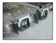
After the exhaust is on the floor, take note of the **mounts** on the stock exhaust, you will see that it is not symmetrical, remove them and install them on the AA exhaust making sure that they are installed in the same configuration.
