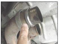
Before installing the AA exhaust, locate the left most pipe on the car and make sure that the "ring" gasket that slides over the pipe is **free to move**.
