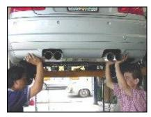
Re-install the 6 valance pins. This should complete the installation
