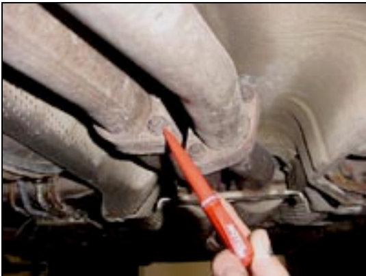
Spray the bolts that hold the exhaust catalyst to the rear muffler. If rusty try soaking first with a rust inhibitor like WD-40 lubricant. -After pulling these bolts the stock M3 exhaust can now be removed.
