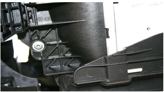
Remove T25 Torx mounting screws on the left and right side of the intercooler.
