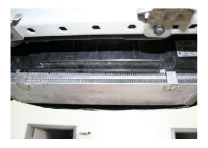
Fit new intercooler into opening aligning factory hoses into intercooler openings and fan shroud into bottom brackets. Due to increased size you may have to have help to stretch spoiler to get intercooler to enter space.
