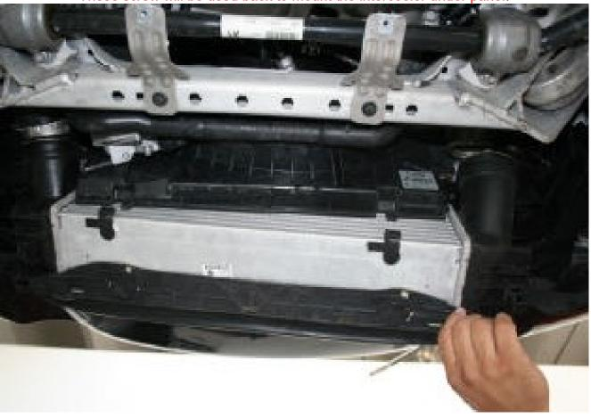
Pull down on intercooler while stretching spoiler to let intercooler pass.
