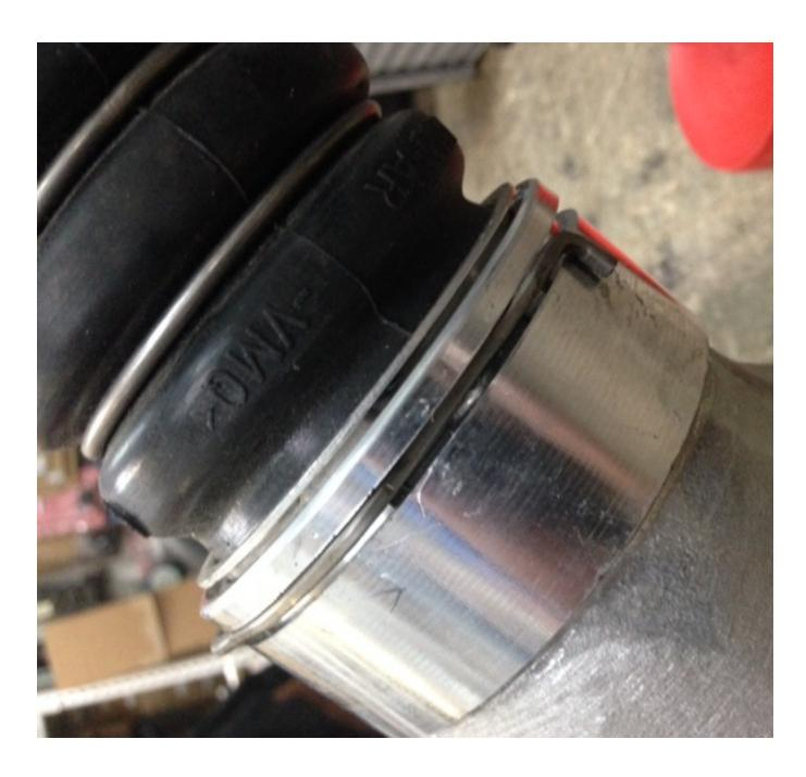
Make sure clip is fully seated in groove.
