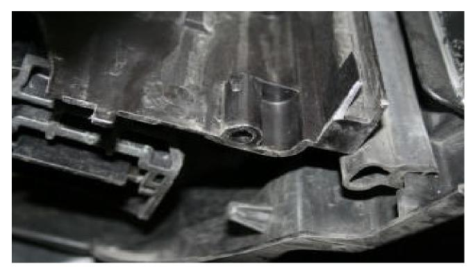
Use back original mounting holes and Torx screws for AA intercooler.
