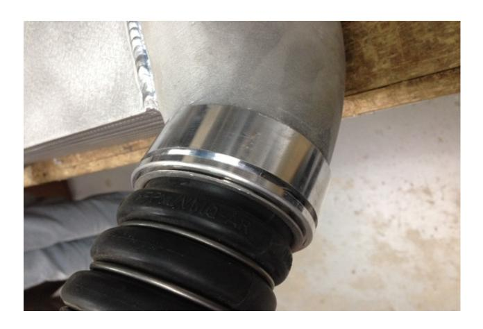
Make sure pipes enter intercooler all the way.
