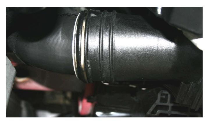
Pull release clips for left and right intercooler pipes. Pull back pipes away from intercooler. May be tight due to rubber O ring.
