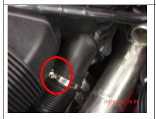
Loosen clamp on front of accordion hose.
