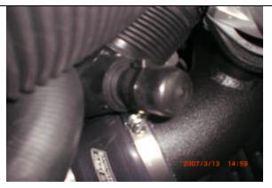
Use rubber caps provided and plug off both holes left by original BOV hoses. Tie strap to secure. These are not under pressure and do not need to be hard clamped.
