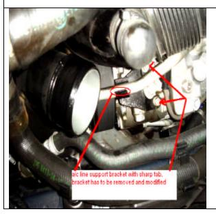
The A/C line support bracket has a sharp edge and can cut into the reducer hose. To prevent it the edge of the bracket must be modified.
