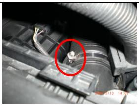
Loosen clamp on accordion hose.
