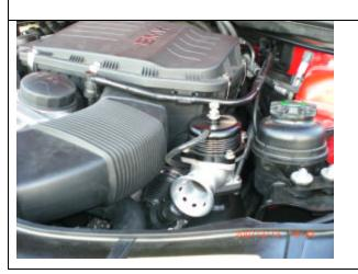
Install back air box, duct and plastic vacuum line. Tighten clamps on the accordion hoses.
