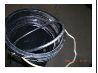
Remove locking clip completely from plastic pipe. Remove O ring from inside the plastic pipe. These have to be reused on the new AA BOV pipe.
