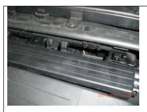
Pull plastic housing that is located against the firewall towards front of car. This will give you a view of the air filter hose (Accordion) at the back.
