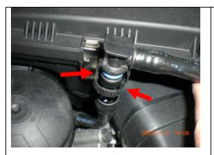
Remove hard plastic line. Squeeze round plastic fitting to release.
