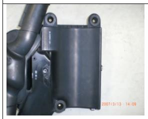
Lift air filter housing up and out. Air filter housing is held down by three grommets.
