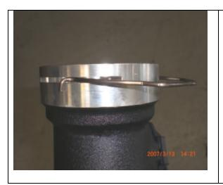
Slide clip half way down the groove on the new BOV pipe.
