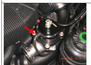
Connect the original vacuum line to the top nipple of the AA BOV.
