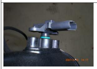
Install sensor into new BOV using the two 4mm blots and washers provided. Sensor plug must face downwards.
