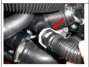
Twist lock and remove both blowoff valve hoses.
