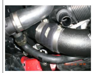
Slide on reducer hose, but do not tighten at this time.
