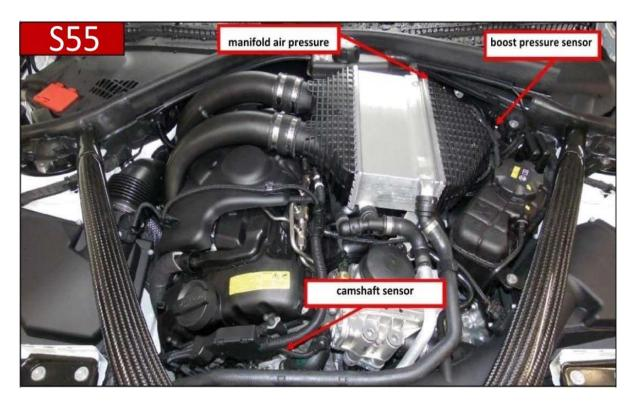
The Active 8 harness will have 3 labeled connectors. Boost pressure sensor, manifold air pressure and the camshaft sensor. On most applications the boost pressure sensor will be before the throttle (usually throttle body or throttle pipe) while the manifold sensor will come after somewhere on the manifold.
