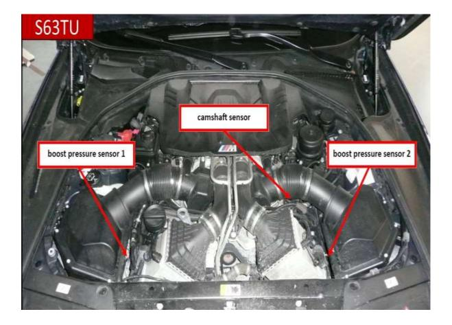
The Active 8 harness has 3 labeled connections: boost pressure sensor 1, boost pressure sensor 2 and the camshaft sensor.
