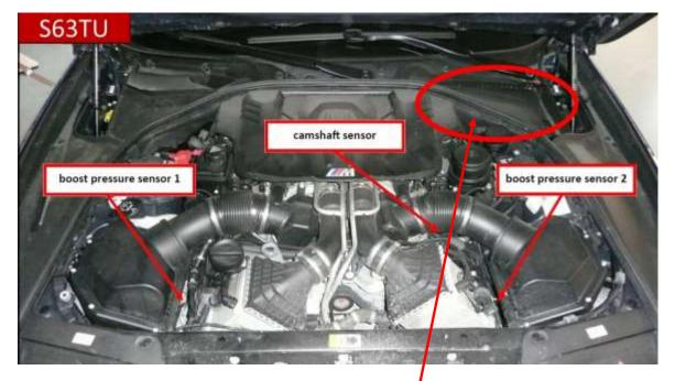
Modules are supplied with an (L) style bracket that is bolted to the large 10mm bolt holding down the Aluminum cross brace.
