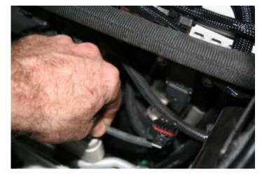
Unlock sensor plug (usually Grey locking tab) and replace with male
