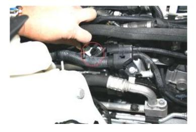
Active Autowerke Software support • Cam sensor ports at back of engine.
