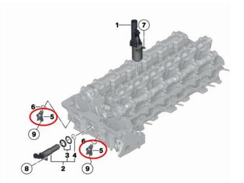
• **Camshaft position sensor:** Unplug the wire from the camshaft position sensor (#5 in diagram)(may require the use of a pick) (since Cam sensor only provides RPM, Intake or Exhaust sensor can be used) plug the Cam sensor harness
