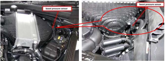
• Manifold air pressure: (Below intercooler coolant bottle) unplug the wire from the manifold sensor (may require the use of a small screw driver or pick) then connect the manifold pressure connector from the Active Module harness.
