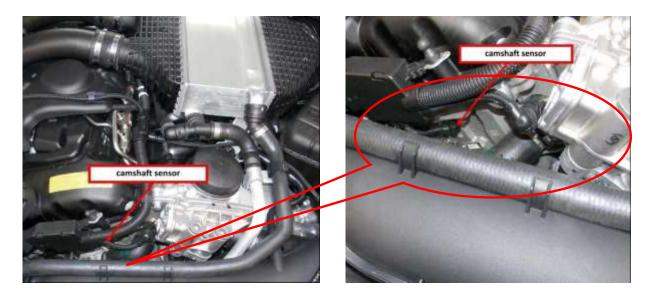
connector into sensor making sure it is fully inserted (only about 5mm of plug should be seen)
