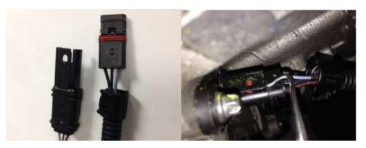
• Before attaching the Active 8 Module, connect Bypass Bridge and start car to make sure harness connections are good. Leave car off for 5 minutes before taking off bridge and attaching module.
