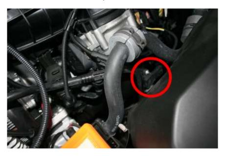
• Unplug Manifold pressure sensor (may require small screwdriver or pick) then connect the manifold pressure connector from Active 8 harness.
