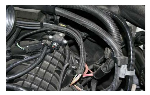
Camshaft position sensor: Unplug the wire from the camshaft position sensor (may require the use of a small screwdriver or pick) plug the cam sensor harness connector into sensor making sure it is fully inserted. (Only about 5mm of plug should be seen). Connect original connector to female leg of Active 8 Cam sensor harness.
