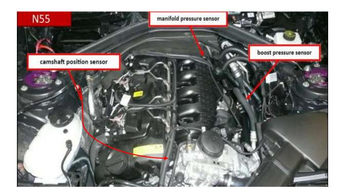
The Active 8 harness has 3 labeled connectors: Boost pressure sensor, manifold pressure sensor and the camshaft position sensor. On most applications the boost pressure sensor will be before the throttle (usually on the throttle body or throttle pipe) while the manifold sensor will come after somewhere on the manifold.
