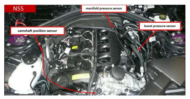
The Active 8 Module use these 3 connections: boost pressure sensor, manifold pressure sensor and the camshaft position sensor. Be aware that the hardness is labeled with the proper connector name, so just follow the label names and connect the hardness connector to each sensor in the engine.
