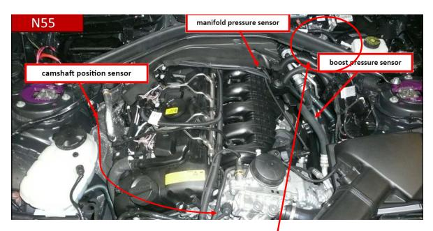
Place the Active 8 Module in the passenger side underneath the highlight section, do not drill a hole there's a hole already, just use the provide bolt.
